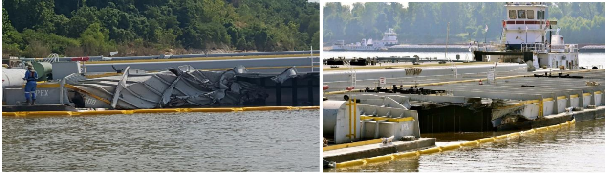
At left, damaged barge APEX 3508 from Dewey R tow; at right, its shell and deck plate have been removed. (Photo by US Coast Guard)
