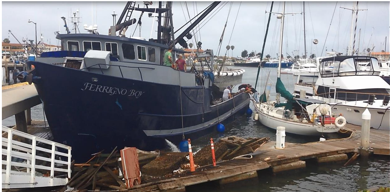
Ferrigno Boy after alliding with the Ventura Harbor Boatyard travel lift pier concrete deck, pilings, and floating docks. (Photo by Ventura Harbor Boatyard)
