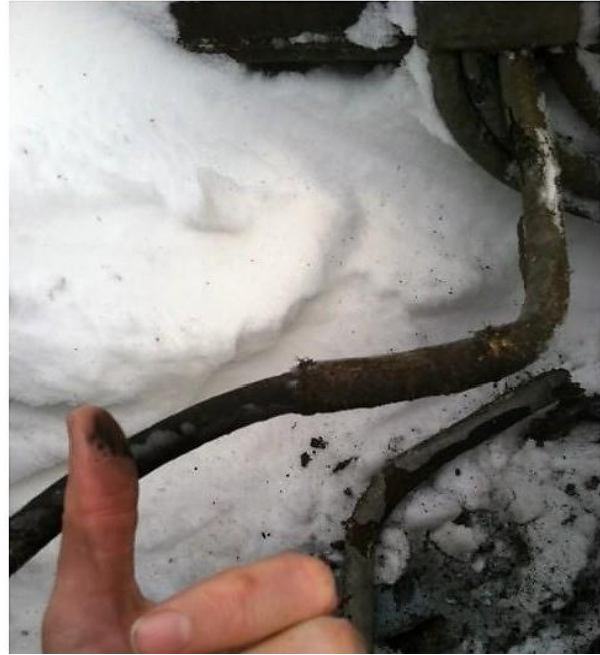
Left, the bundled wires running from the electrical control panel to the aft anchor winch. Right, the outer sheathing of the wire in its decayed and deteriorated condition. (Photos by Coast Guard)
