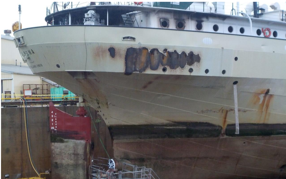
Alpena with fire damage to the hull paint on the starboard quarter and burned-out portholes on the superstructure. (Photo by Coast Guard)
