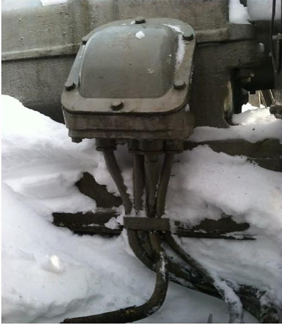
Left, the bundled wires running from the electrical control panel to the aft anchor winch. Right, the outer sheathing of the wire in its decayed and deteriorated condition. (Photos by Coast Guard)
