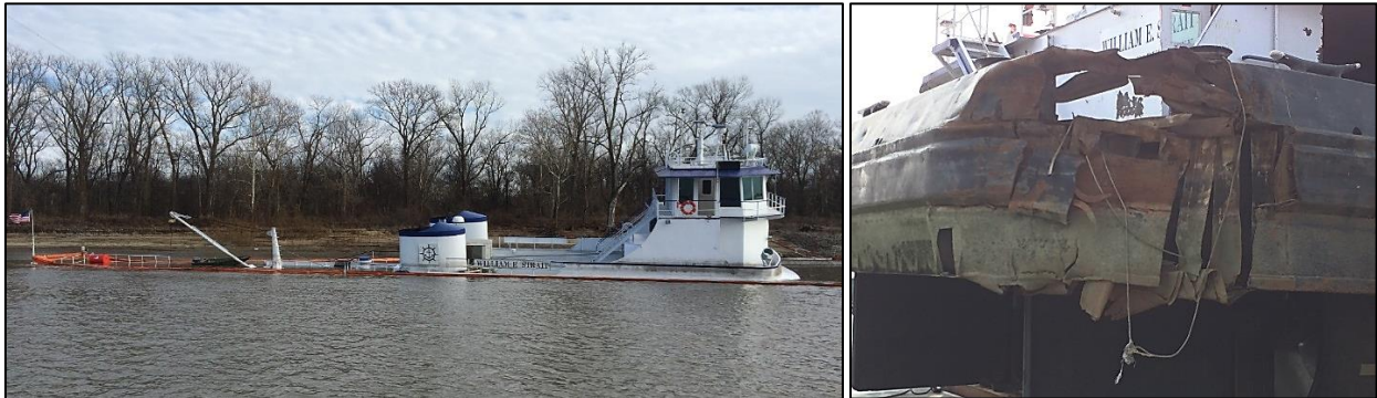
Left image is of the partially submerged William E Strait taken shortly after the collision. The wheelhouse, exhaust stacks, davit system, and aft flag staff are seen above the surface of the river. Right image, taken after the vessel was salvaged, is of the damaged hull near the starboard stern.
