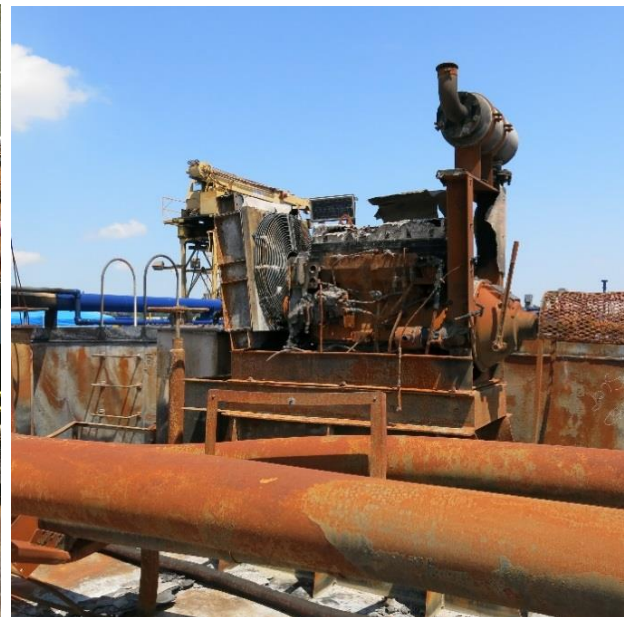
EMS 343 after the accident: at left, fire damage on outboard side; at right, burned diesel engine.
