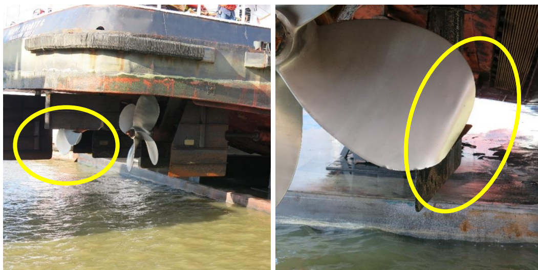
Stern of Capt. Shorty C in drydock: at left, circled in yellow, missing lower portion of the starboard rudder; at right, bent fluke of the port propeller.
