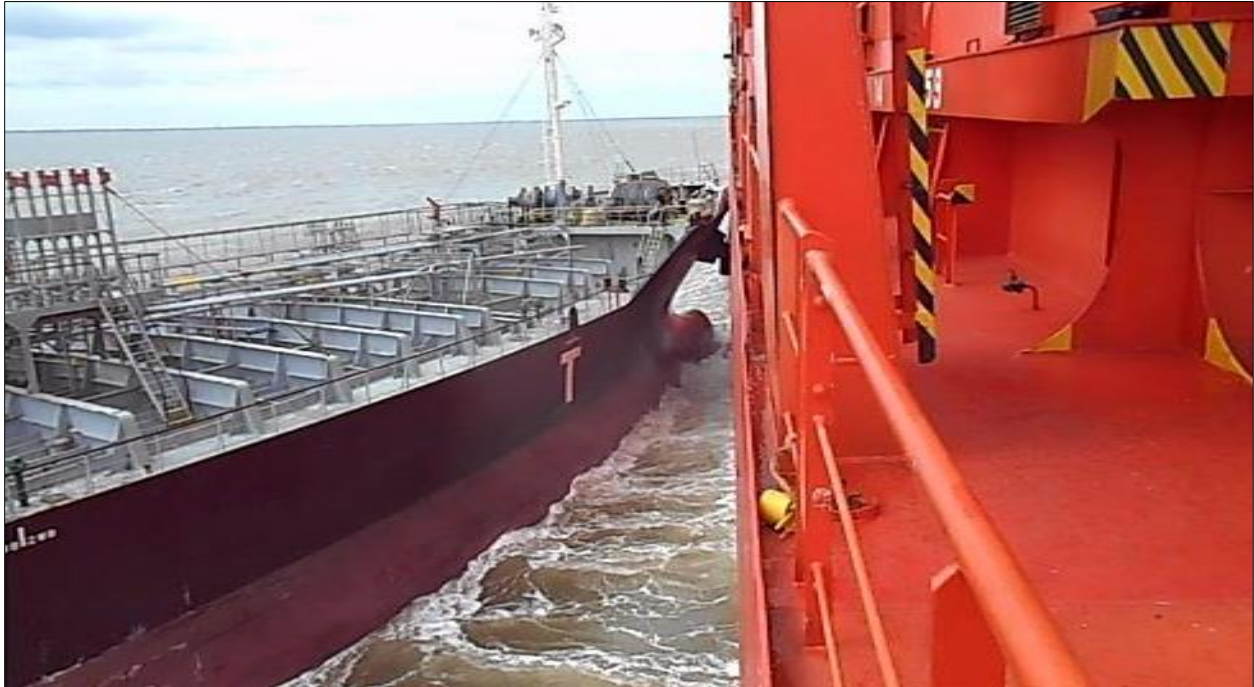
Still image extracted from video on board the Monte Alegre , showing the Chembulk Houston 's starboard-side bow and anchor in contact with the Monte Alegre 's port side. The initial contact occurred farther aft on the Monte Alegre .
