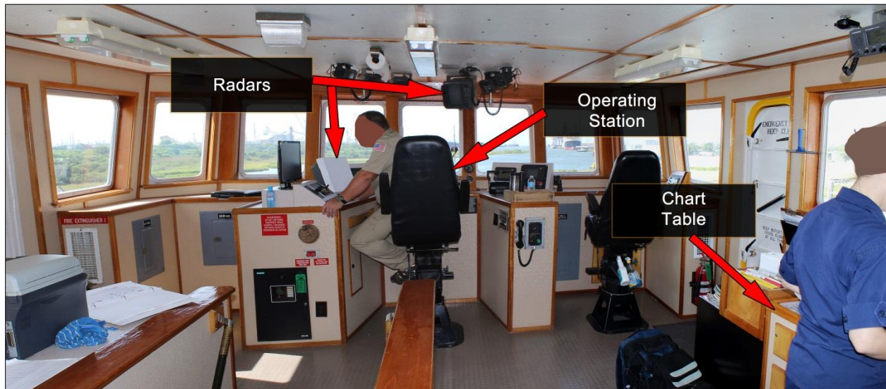
Wheelhouse of the Gloria May , looking from aft to forward at centerline. The operating station is at the forward area of the wheelhouse, and the chart table is at the starboard side.
