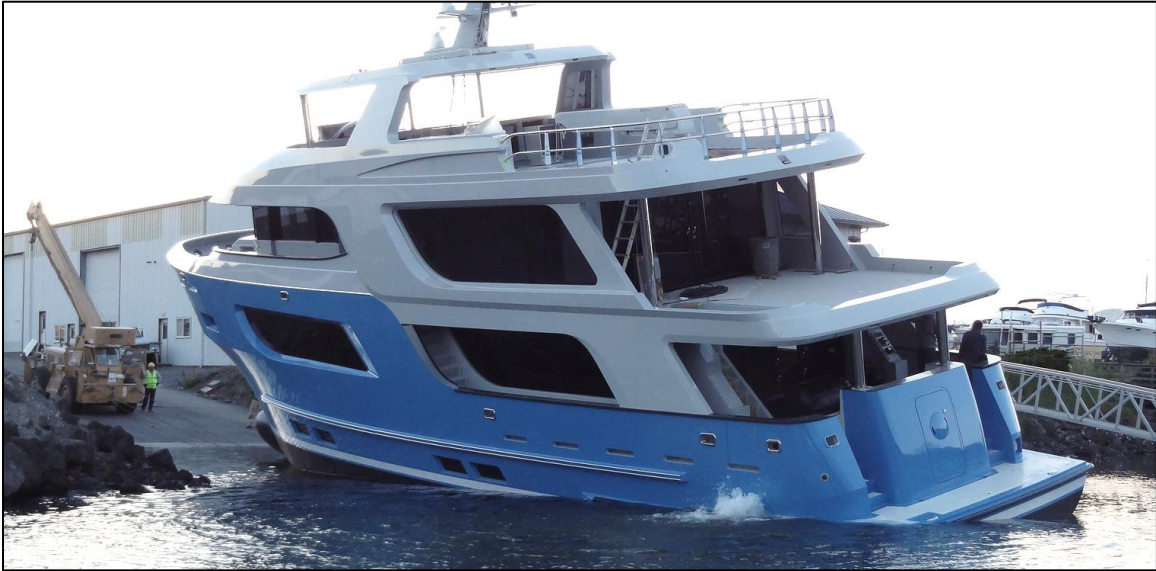
The Baaden after its initial roll to port and stable at about 12 degrees with its generators and propulsion engine running. (Photo provided by Western Mariner )
