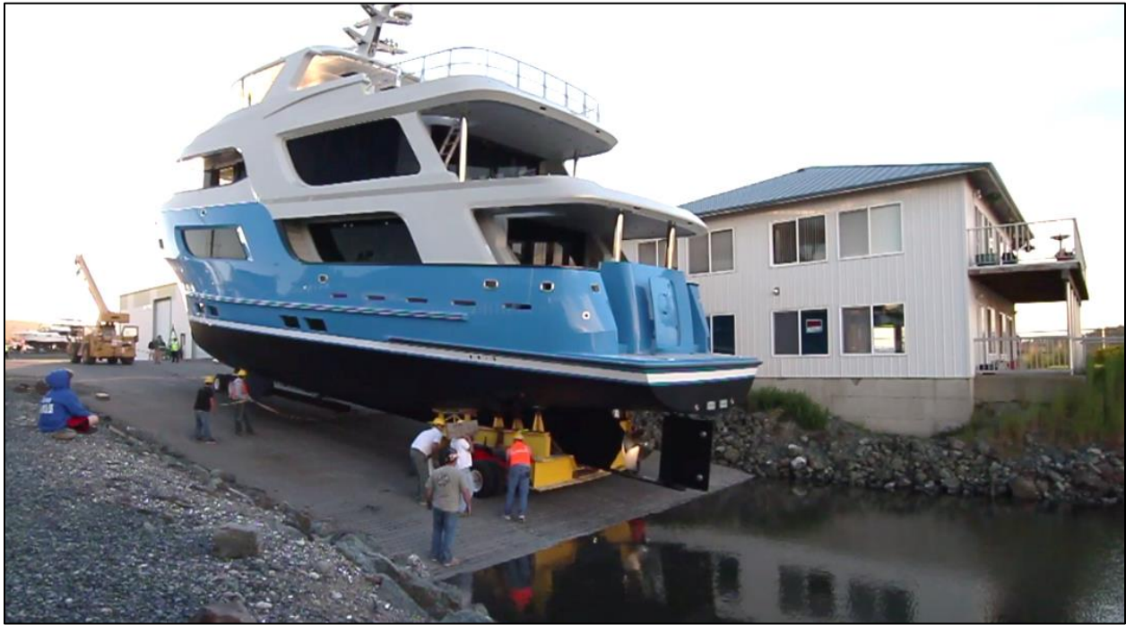
The Baaden on its front and rear dollies on the upper ramp prior to final launching. (Photo from YachtVid video)
