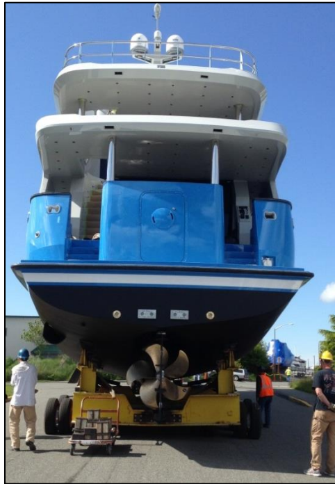
Stern view of Baaden and aft dolly during the vessel's tow toward the launch ramp. (Photo by New World Yacht Builders)
