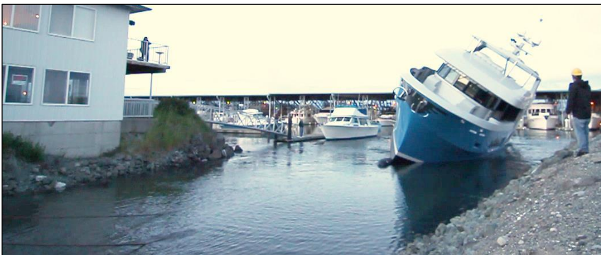
The Baaden at 25 degrees port heel (determined by NTSB video study) and in the process of rolling completely over to port while backing down. (Screenshot from YachtVid video)
