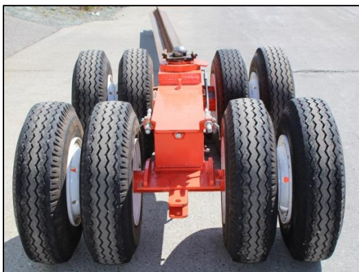
Front dolly with connecting bar (left) and the two rear dollies and aft cradle assembly (right). (Photos by Coast Guard)
