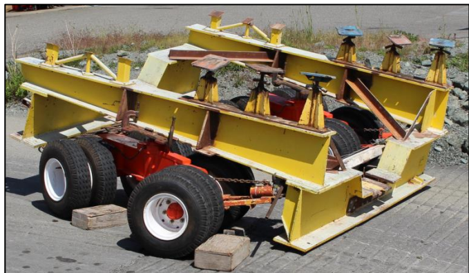
Front dolly with connecting bar (left) and the two rear dollies and aft cradle assembly (right). (Photos by Coast Guard)
