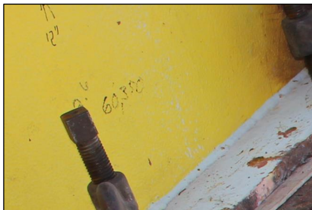
Left, aft starboard load cell reading of 60,550 pounds taken in March 2015. (Photo by New World) Right, aft starboard cradle grease pencil marks indicating 60,350 pounds 2 days after the accident. (Photo by Coast Guard)
