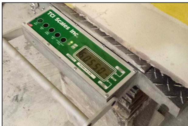
Left, aft starboard load cell reading of 60,550 pounds taken in March 2015. (Photo by New World) Right, aft starboard cradle grease pencil marks indicating 60,350 pounds 2 days after the accident. (Photo by Coast Guard)
