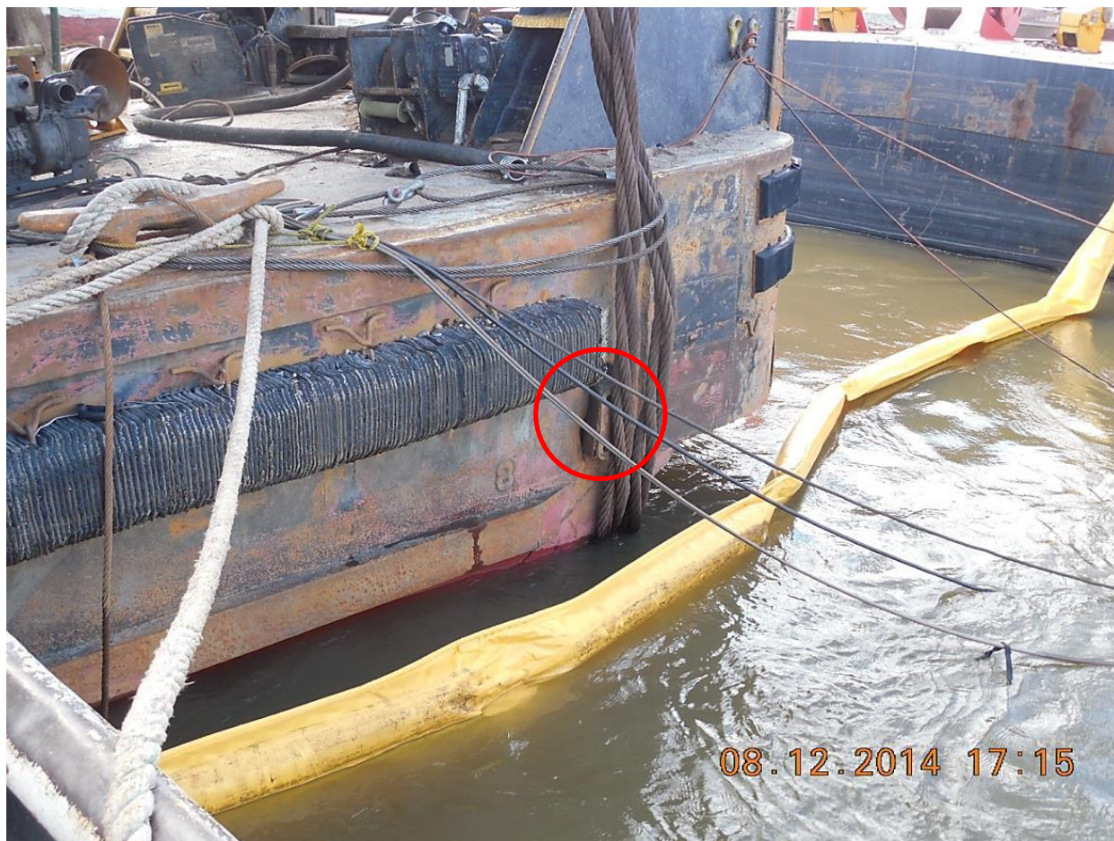
Postsalvage photo of the starboard bow area. The hole created by the gusset bracket is circled in red. (Photo by the Coast Guard)
