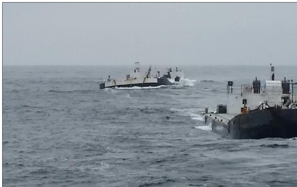
Barges Nash (left) and Kenny under tow on the afternoon of the accident. The Nash is heeled to its starboard side. (Photo by Salmon Bay Barge Line)
