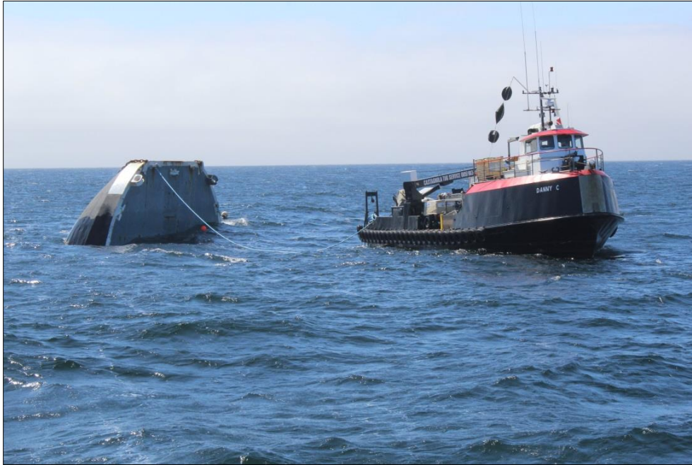
Dive boat Danny C (right) engaged in salvage operations of the Nash and the bow of the Nash (left) protruding vertically about 15 feet above the sea.
