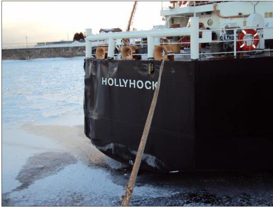
Damage to the left side of the cutter Hollyhock 's stern, where the steel was inset and displaced by the force of the collision with the bow of the Mesabi Miner .
