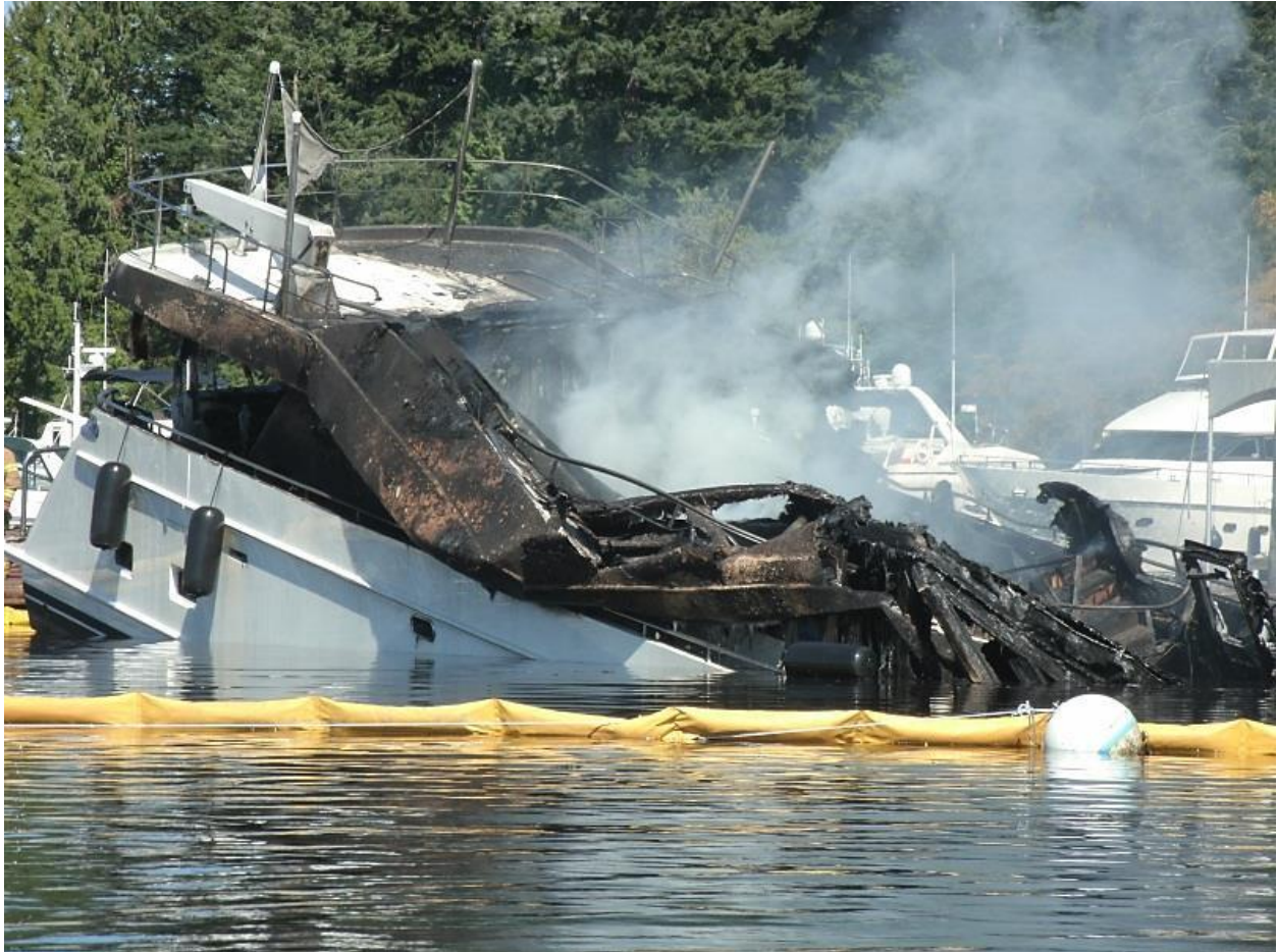
The starboard side of the Ocean Alexander 85E06 after the fire was extinguished. The stern is visible and the bow has sunk below the water. The pollution prevention boom can be seen in the foreground. (Photo by the Coast Guard)
