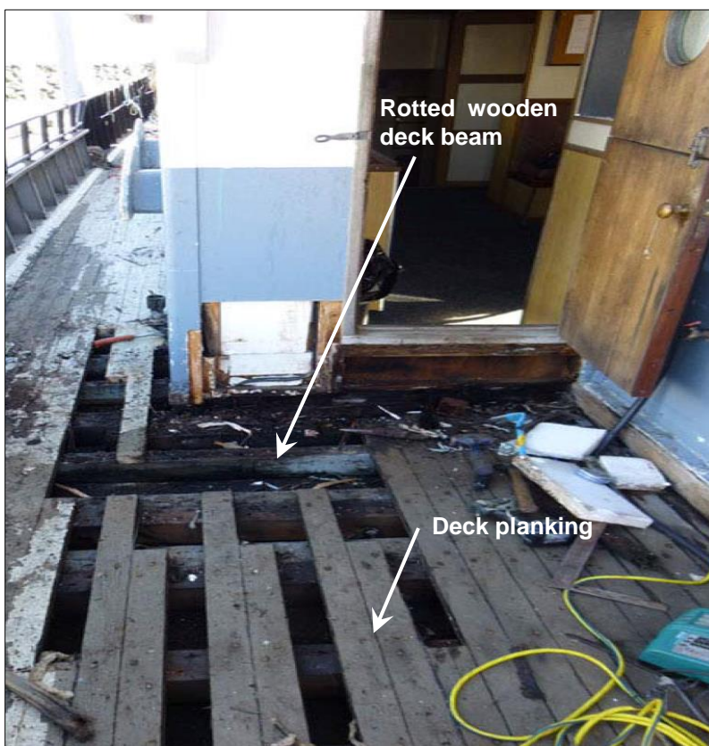
Moonlight Maid portside deck under repair, Seward Dock, September 2012. The top arrow indicates an area of rot found in structural member. (Photo provided by Coast Guard Sector Anchorage)
