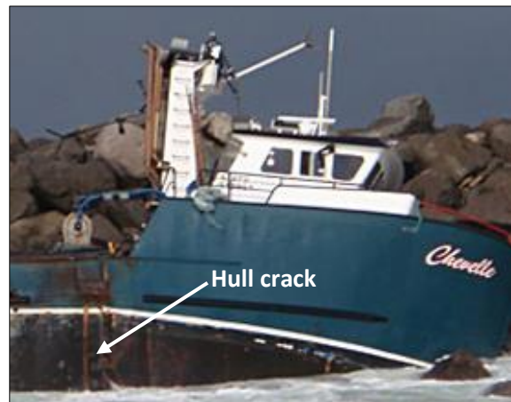
Chevelle against the rocks of the north jetty with arrow pointing to crack in hull. (Photo by Coast Guard)
