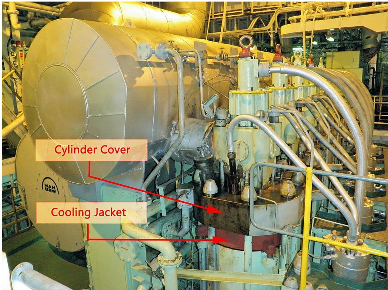
The *FR8 Pride*'s main propulsion engine, with the location of the failed engine component (cooling jacket for cylinder No. 5) indicated. Photo by the Coast Guard.
