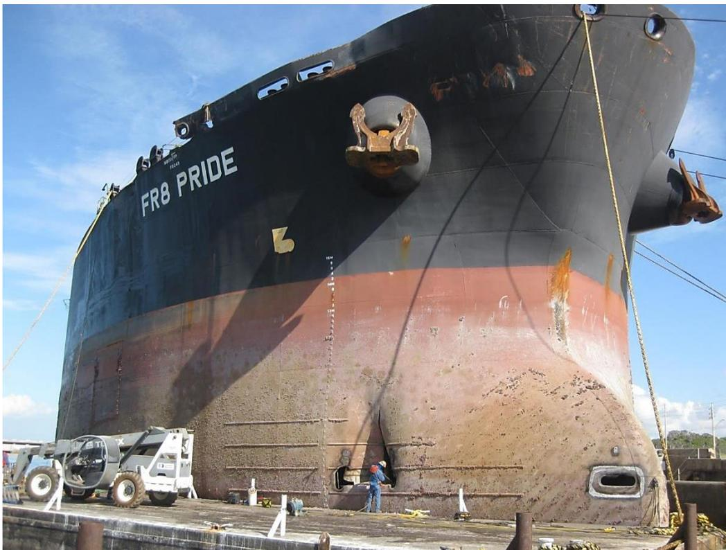
Damage to the *FR8 Pride*, including the puncture to the hull below the waterline, visible in the lower center of the image. Photo provided by the Coast Guard.
