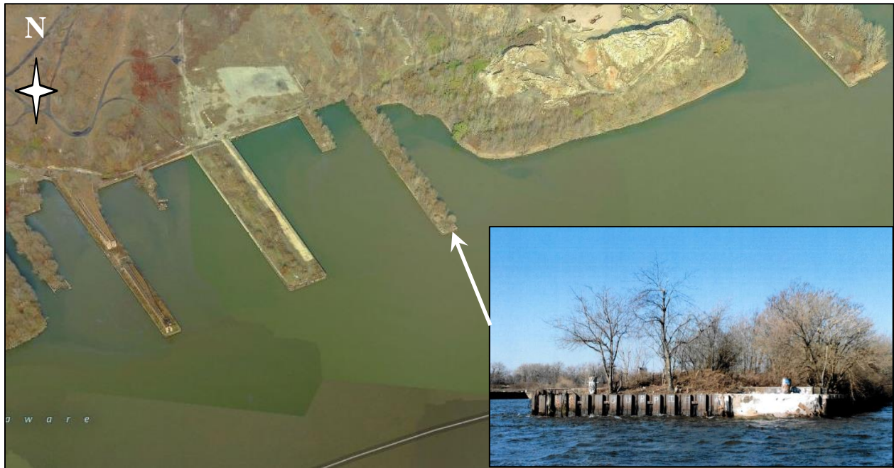
Birdseye view of Pier 11 vicinity with inset image showing the damage to the southeast corner of Pier 11's corrugated steel pilings. The area on the right side of the pier that appears white is damage due to the allision.
