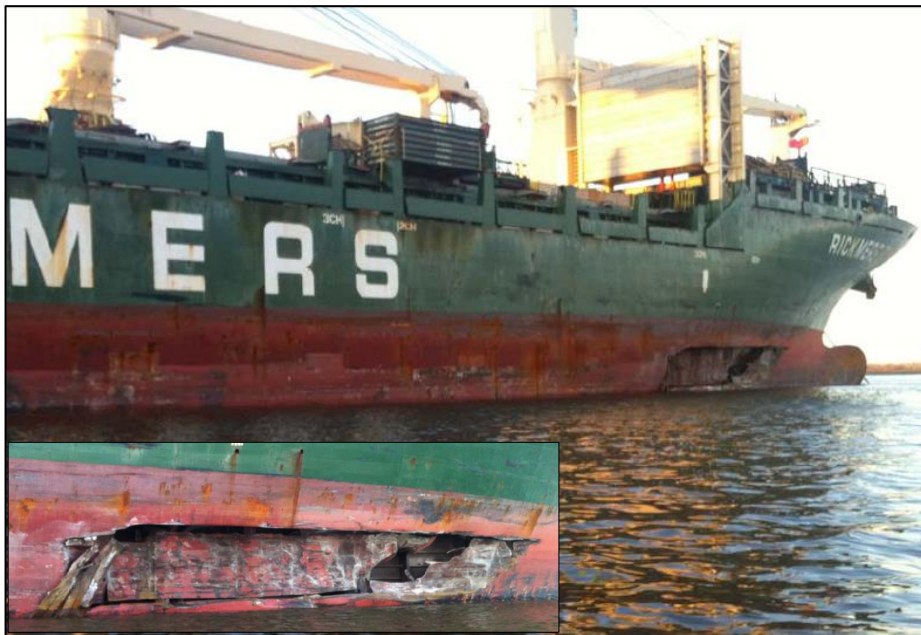
Starboard side damage to the Rickmers Tokyo , with inset image showing close-up of sheet steel piling stuck in the aft portion of the hull penetration.
