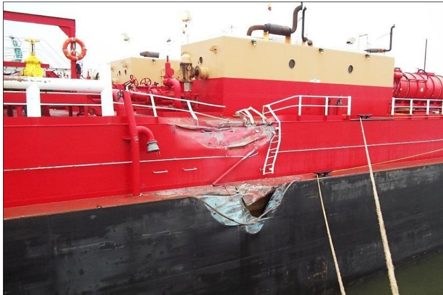
Portside damage to the RTC 102 .
