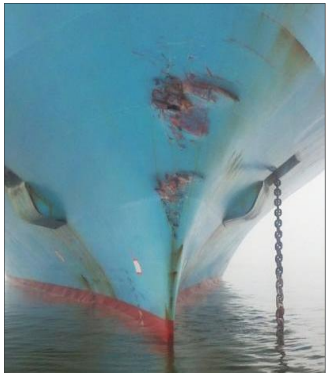
Damaged bow of the Maersk Wisconsin . Photo by US Coast Guard
