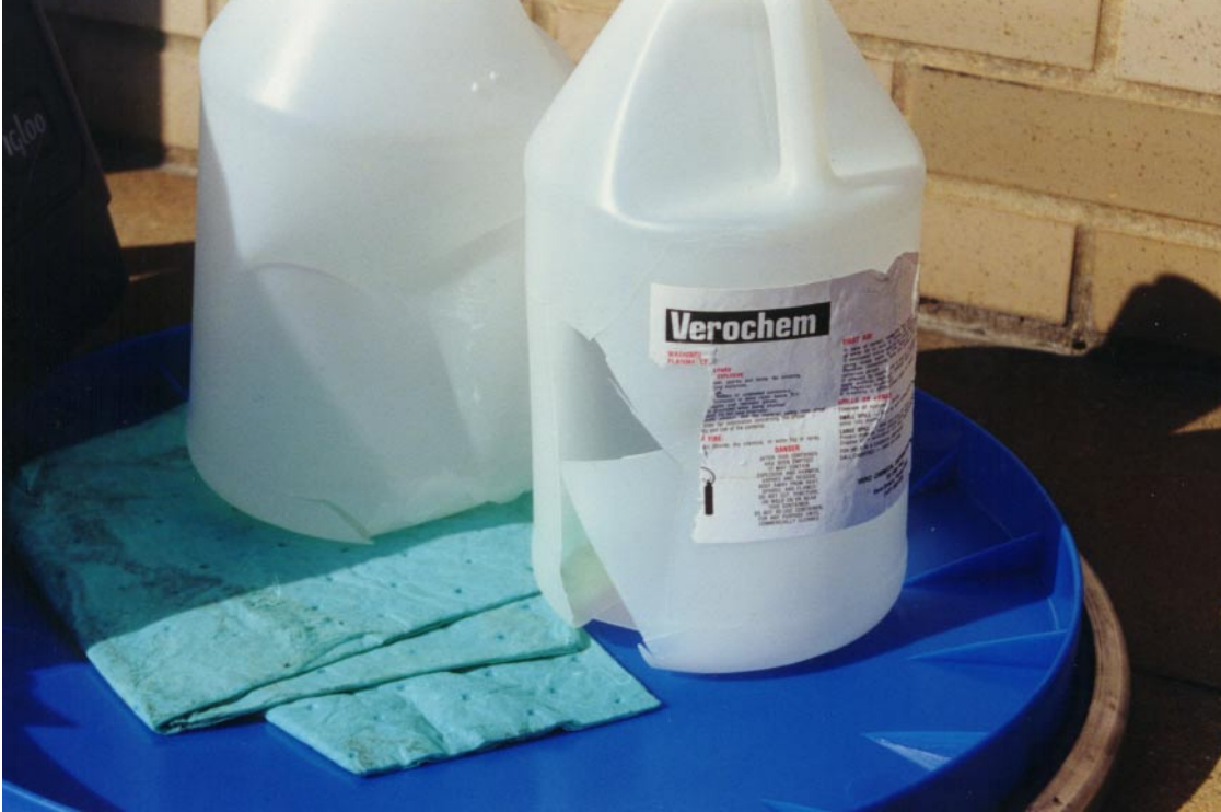
Figure 2. Damage to the bottles of hydrogen peroxide.
