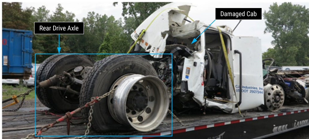
Figure 8. Photo of the crash-damaged Mack truck-tractor, viewed from the front left. During recovery, the truck-tractor’s separated rear drive axle was located and secured in front of the damaged cab.
