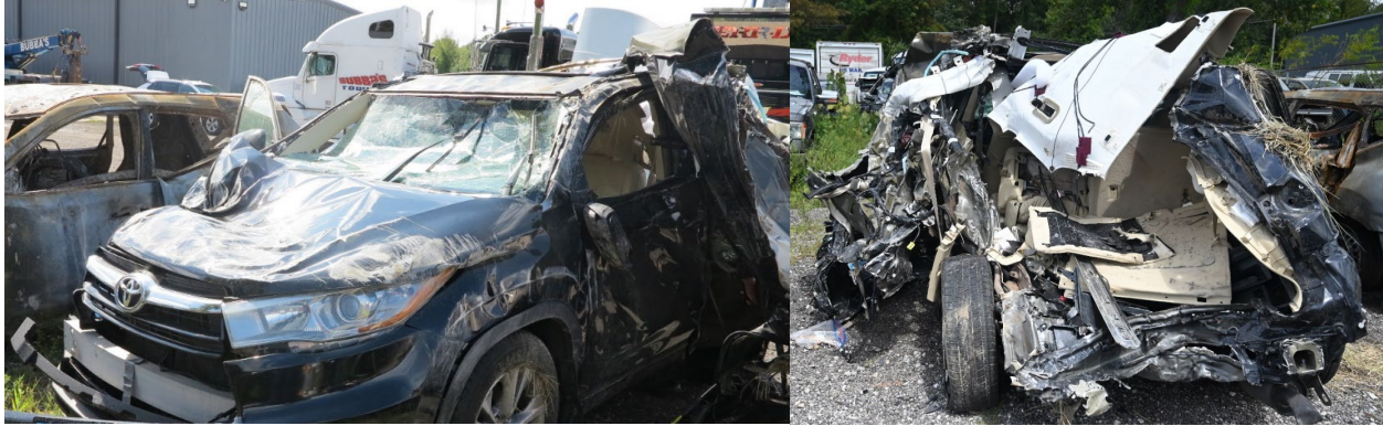
Figure 9. Photo of the front (left image) and rear (right image) of the crash-damaged SUV.
