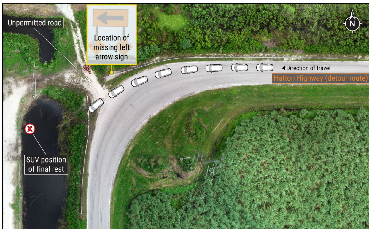
Figure 4. Reconstructed overhead image of the SUV's travel path to impact location. (Source: Google Earth; inset image and annotations by NTSB)
