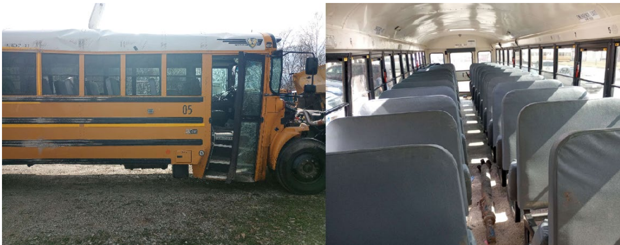
Figure 5. Damage to the bus's right (loading door) side; an interior photograph showing lack of intrusion into the passenger compartment. (Source: WVSP)
