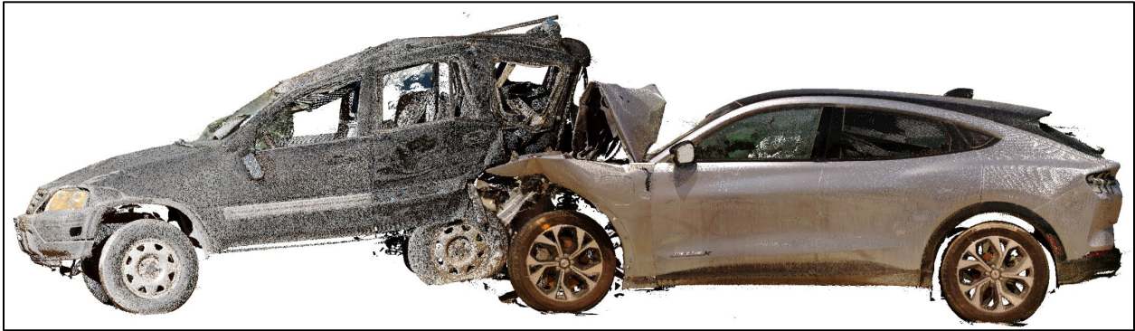
Figure 20. Side-view image of the alignment of vehicle laser scans illustrating the likely maximum engagement of the Ford (right) and Honda (left) during the crash.
