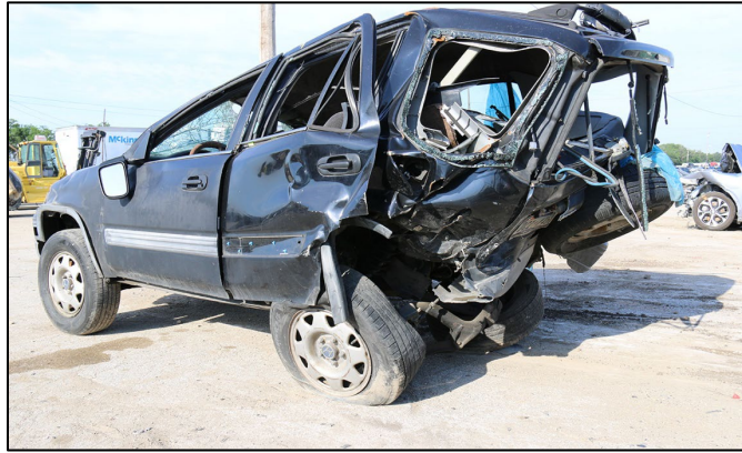
Figure 10. Rear left view of damage to the Honda.
