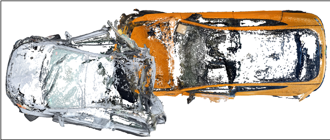
Figure 21. Overhead image of the alignment of vehicle laser scans illustrating the likely maximum engagement of the Ford (right) and Elantra (left) during the crash.
