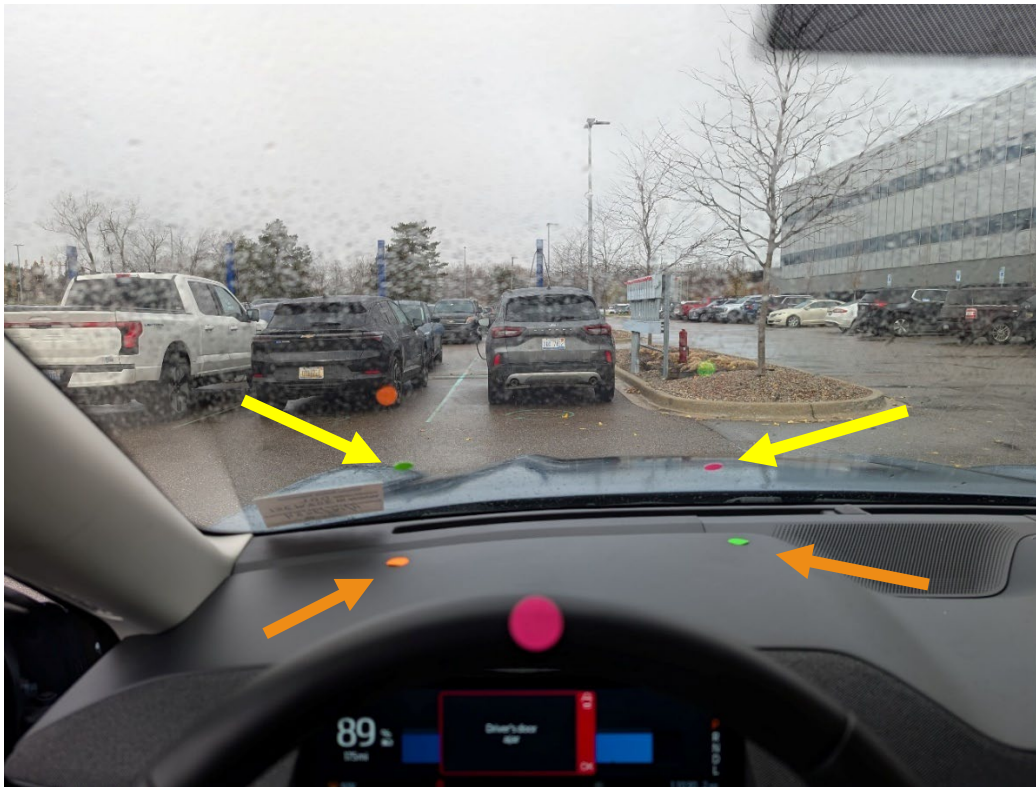
Figure 26. Fixation locations targeted by the exemplar driver. The two markers highlighted by yellow arrows are within the Front Windshield gaze zone, and the two markers highlighted by orange arrows are outside this zone. The pink marker on top of the steering wheel was obscured by the cell phone during the with-phone conditions. (Note: The apparent additional markers above the yellow arrows are reflections of the bottom markers.)
