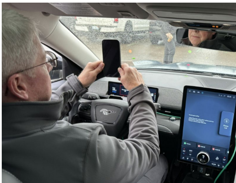
Figure 25. Forward-facing view of exemplar driver in the vertical phone test condition.
