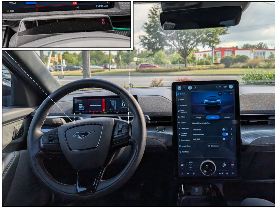
Figure 3. Ford Mach-E interior DMS camera (inset) and instrument cluster.
