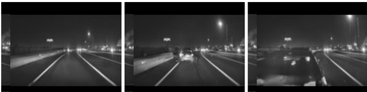
Figure 15. Enlarged versions of the images captured by the forward-facing camera at 1-Hz intervals, from 2 seconds precrash to the point of impact.
