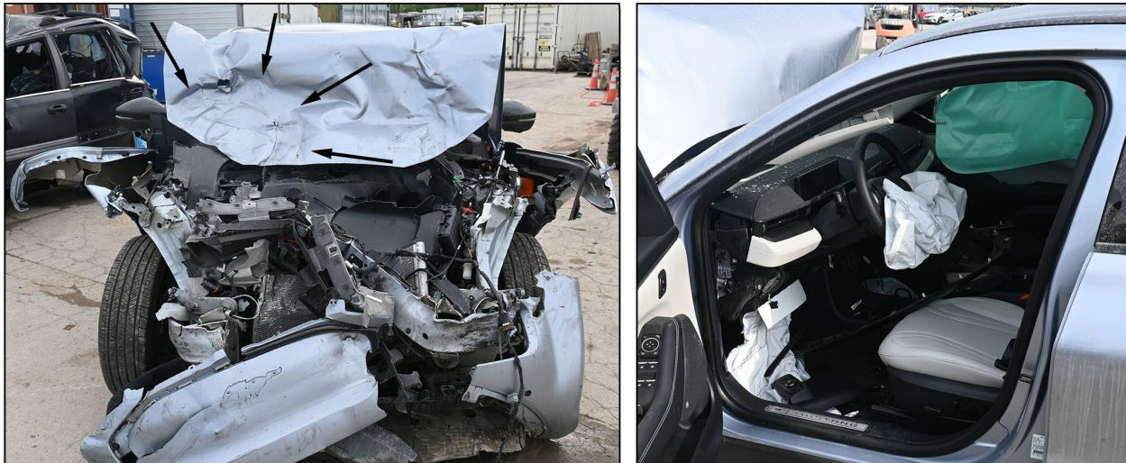
Figure 6. Left: Front view of damage to the Ford with the Honda's spare tire marking indicated by arrows. Right: View of the interior of the Ford.
