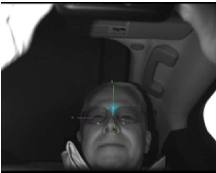
Figure 24. Driver-facing DMS live-image feed view of the exemplar driver in the vertical phone test condition.
