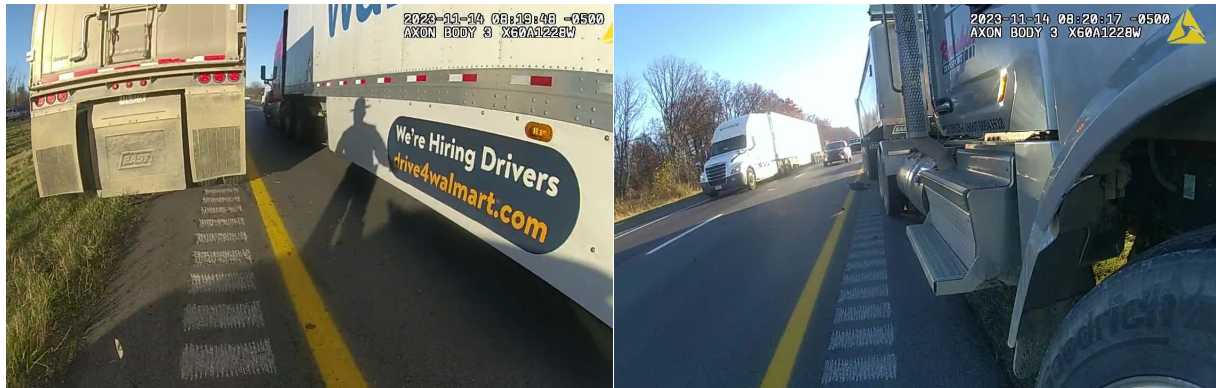
Figure 8. Trooper body camera images showing locations of vehicles from initial crash after they were moved to the median. The right rear of the trailer involved in the initial crash was nearly on the solid yellow edge line and inches away from traffic traveling in the left lane of westbound I-70. (Source: OSHP)
