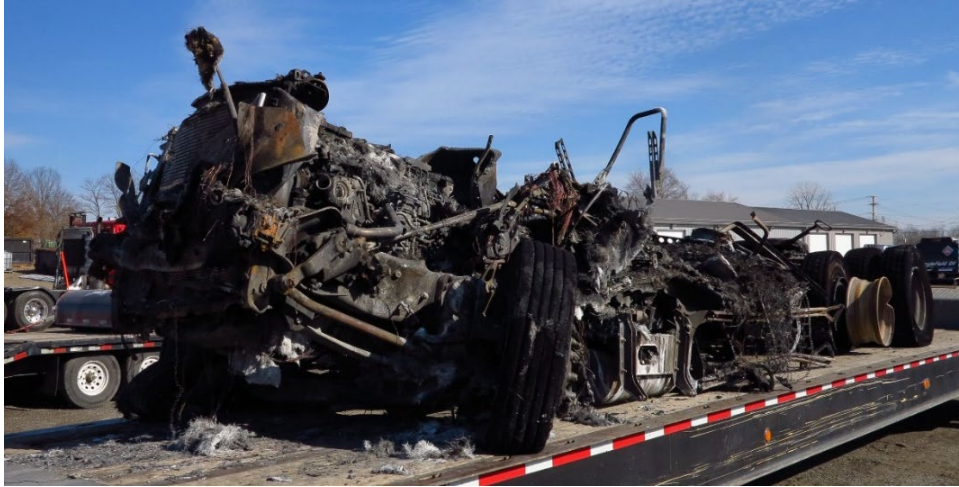
Figure 10. Damage to Freightliner truck-tractor.
