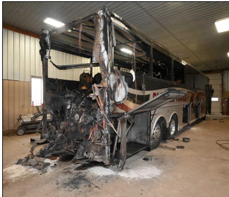
Figure 11. Damage to right rear of motorcoach.
