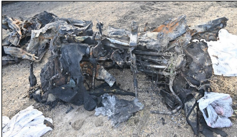
Figure 13. Postcrash view of Nissan, which sustained catastrophic crash damage and comprehensive fire damage.
