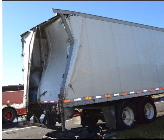
Figure 15. Damage to rear of Volvo combination vehicle Vanguard semitrailer. (Source: OSHP)
