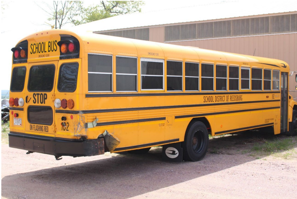
Figure 4. Postcollision photograph of the 2016 Blue Bird school bus showing damage to the right-rear corner. (Source: NTSB)
