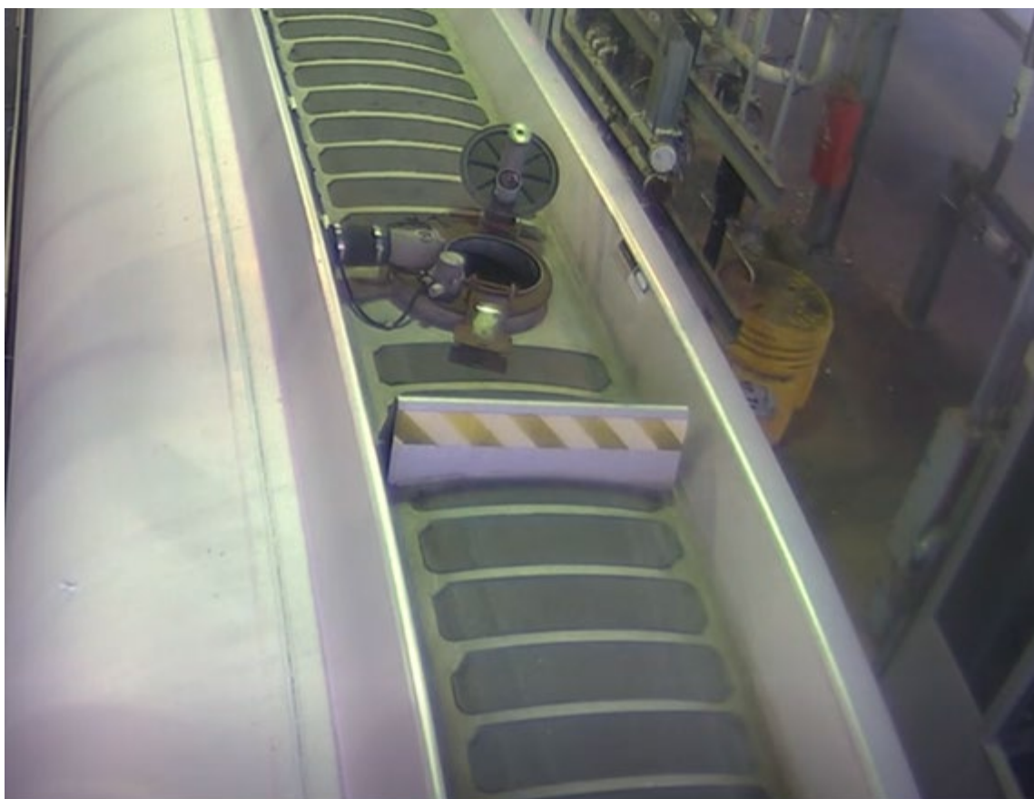
Figure 5. Loading facility video footage showing open manhole cover atop cargo tank. (Source: Buckeye Terminal, Wilmington, Delaware)
