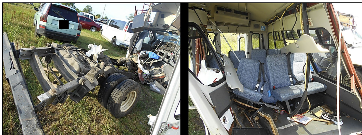
Figure 5. Damage to the bus, showing the detached chassis (left) and the interior intrusion (right).
