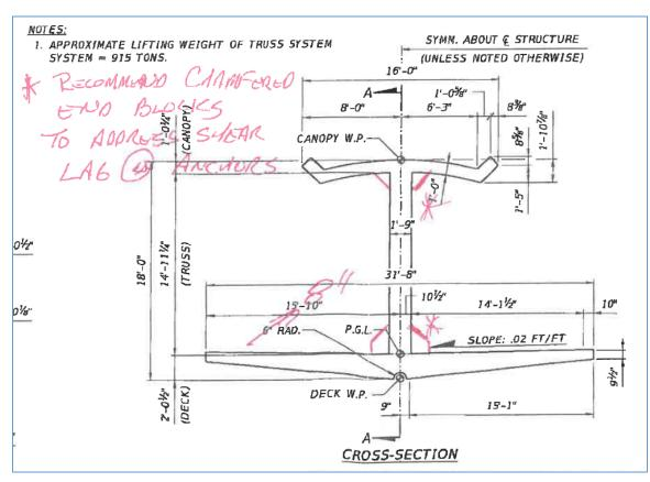
**Figure 28.** FDOT comments to FIGG on main span truss system layout, recommending chamfered end blocks to address shear lag at anchors. (Source: FDOT)
