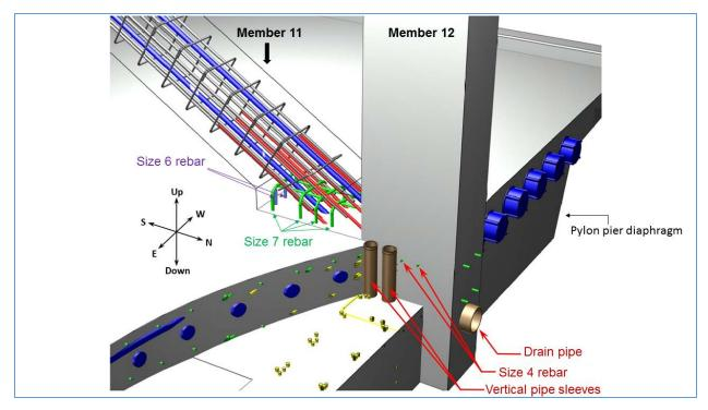
**Figure 16.** Main span, north end, showing steel rebars in member 11, vertical pipe sleeves, end of drain pipe location, and size 4 rebar at member 12. (Source: FHWA 2019)
