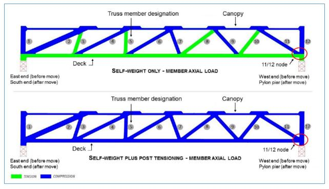
**Figure 21.** Self-weight axial forces only (top) for diagonal truss members 2 and 11, which are combined with post-tensioning forces concurrently acting on main span to produce net axial forces (bottom) at each end before transport and on permanent pier following transport. Top illustration is shown without post-tensioning; bottom illustration is shown with actual loads. (Source: FIGG, annotated by NTSB)
