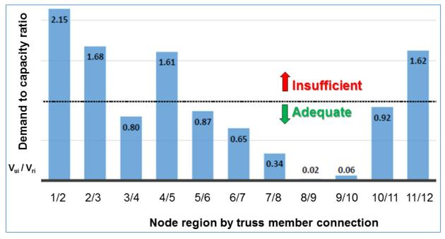
Figure 31. D/C ratios for main span nodal regions. (Source: FHWA 2019)
