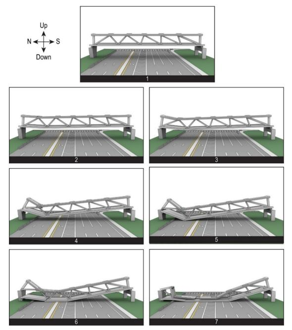
**Figure 12.** Collapse sequence diagram, facing east, depicting bridge's precollapse condition in phase 1 through postcollapse position (onto SW 8th Street) in phase 7.
