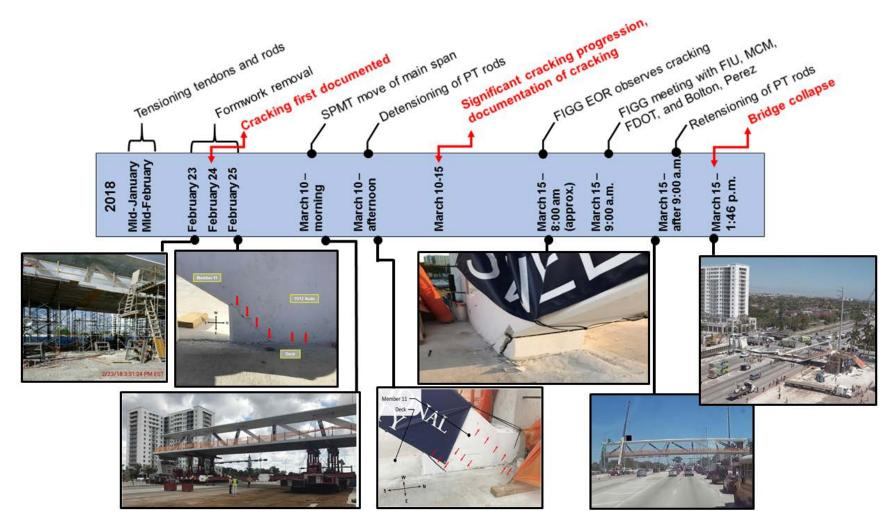
Figure E-1. Timeline of precollapse events.
