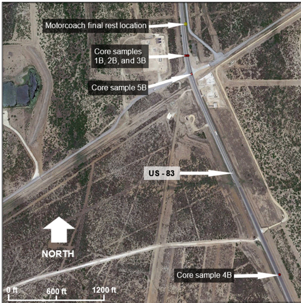
Figure 10. Locations on US-83 where the pavement core samples were obtained. (Source: Google Earth modified)
