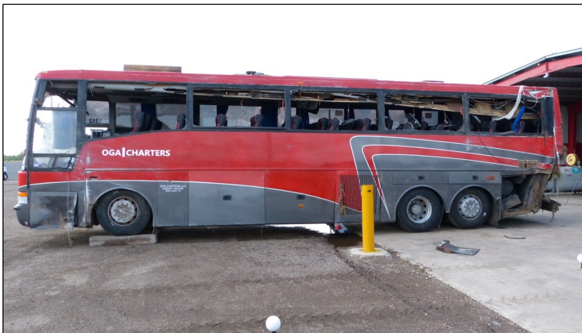
Figure 6. View of motorcoach's left side, showing missing window panes and impact damage to the front and rear of the vehicle.
