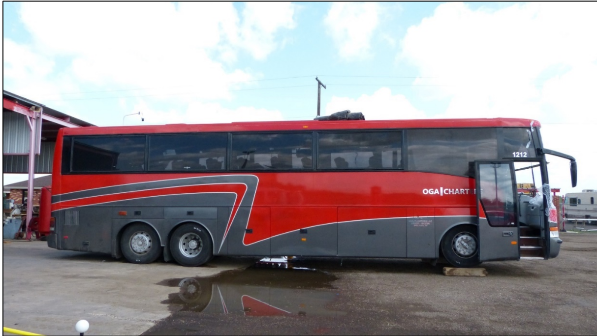
Figure 7. View of motorcoach's right side, showing intact window panes and minimal vehicle damage.
