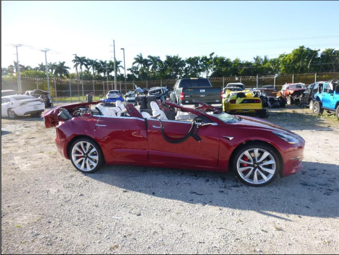
Figure 5. Right side of car in postcrash damaged condition.
