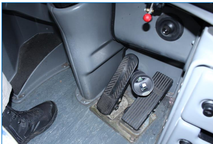
Figure 3: Pedal obstruction test using exemplar motorcoach and metal thermos, showing one lodging position among several possible thermos and pedal combination scenarios.
