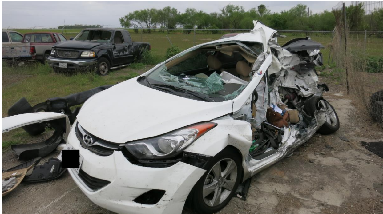
Figure 2. Wreckage of the 2013 Hyundai Elantra.
