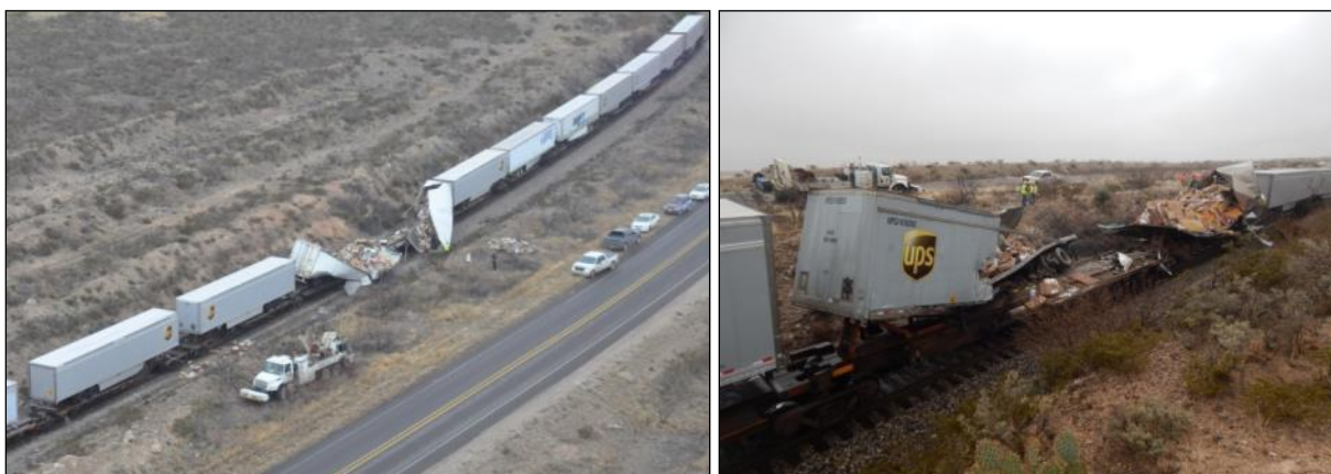
Figure 7. At left, two damaged semitrailers on intermodal flatcar. At right, closer view of damaged semitrailers. (Source: TxDPS)
