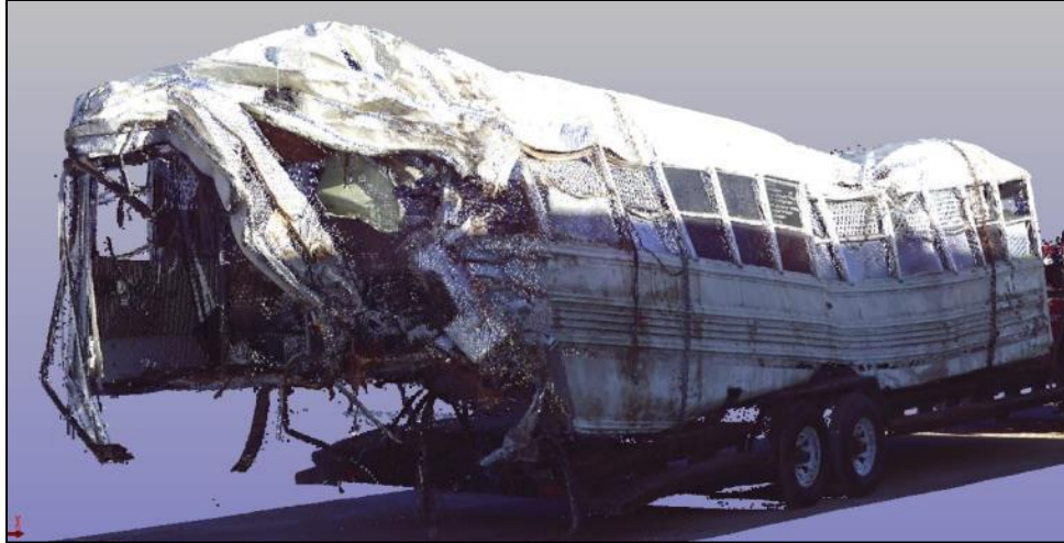
Figure 6. 3D scan showing damage to front, roof, and left side of bus body, which is resting on a tow vehicle.
