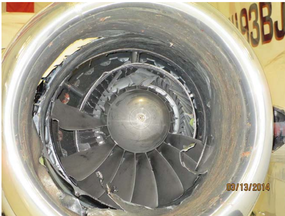
Figure 3. Photograph showing damage to the inlet cowl of the No. 2 engine on N193BJ.
