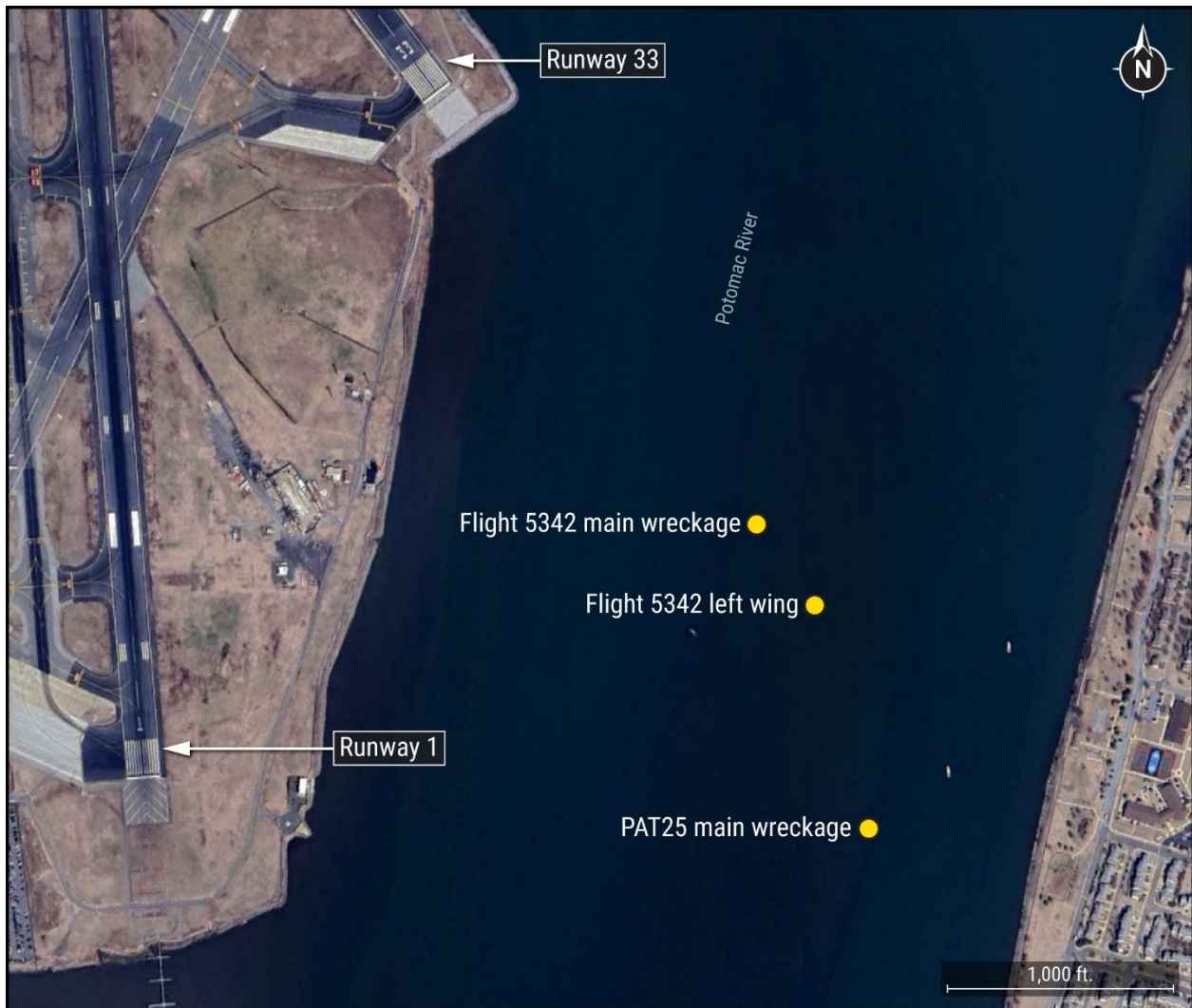
Figure 26. Diagram of main wreckage locations in the Potomac River.
