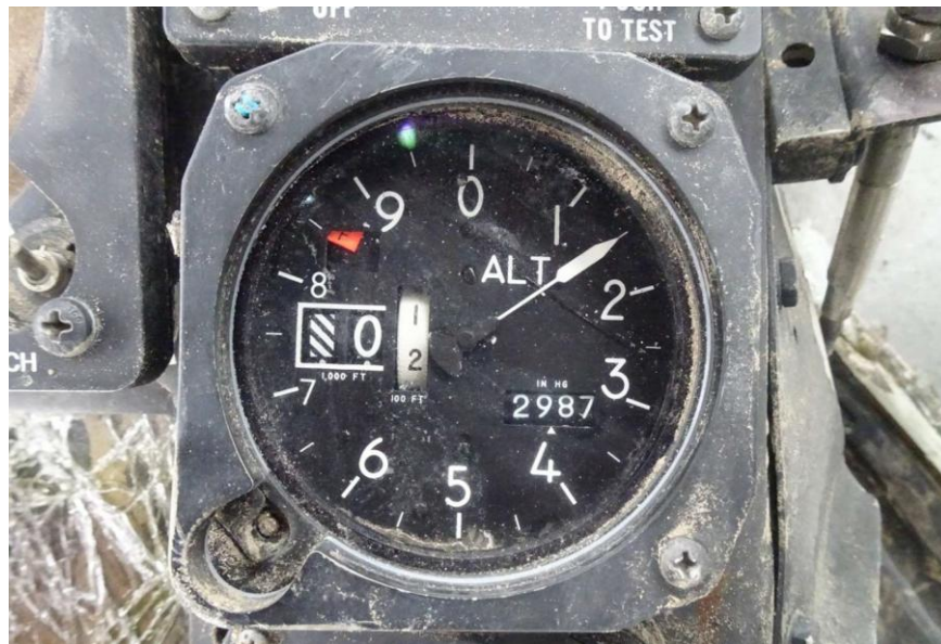
Figure 34. The right (IP's seat) barometric altimeter.
