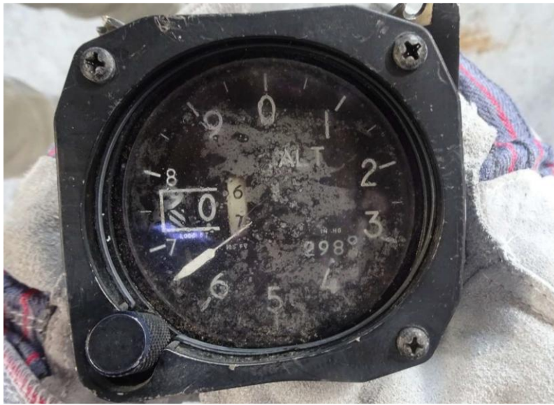
Figure 33. The left (pilot's seat) barometric altimeter.
