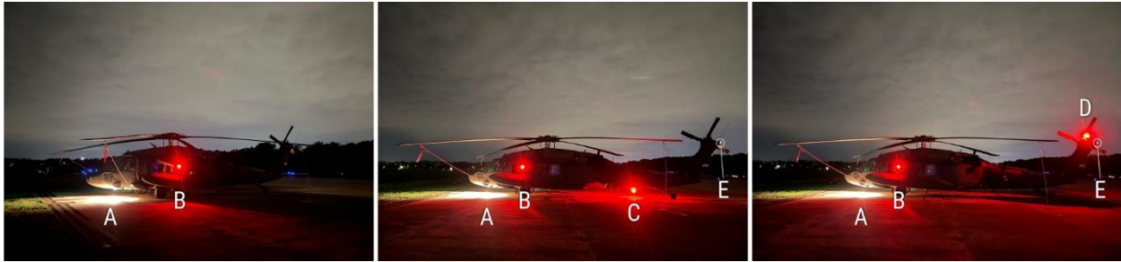
Figure 38. Left view of a UH-60L showing landing light (A), left navigation light (B), flashing lower anti-collision beacon (C), flashing upper anti-collision beacon (D), and tail position light (E).
