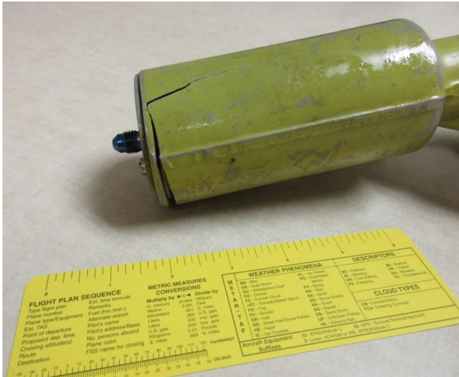
Figure 1. Actuator with fatigue cracking (from NTSB case number ANC18LA019).
