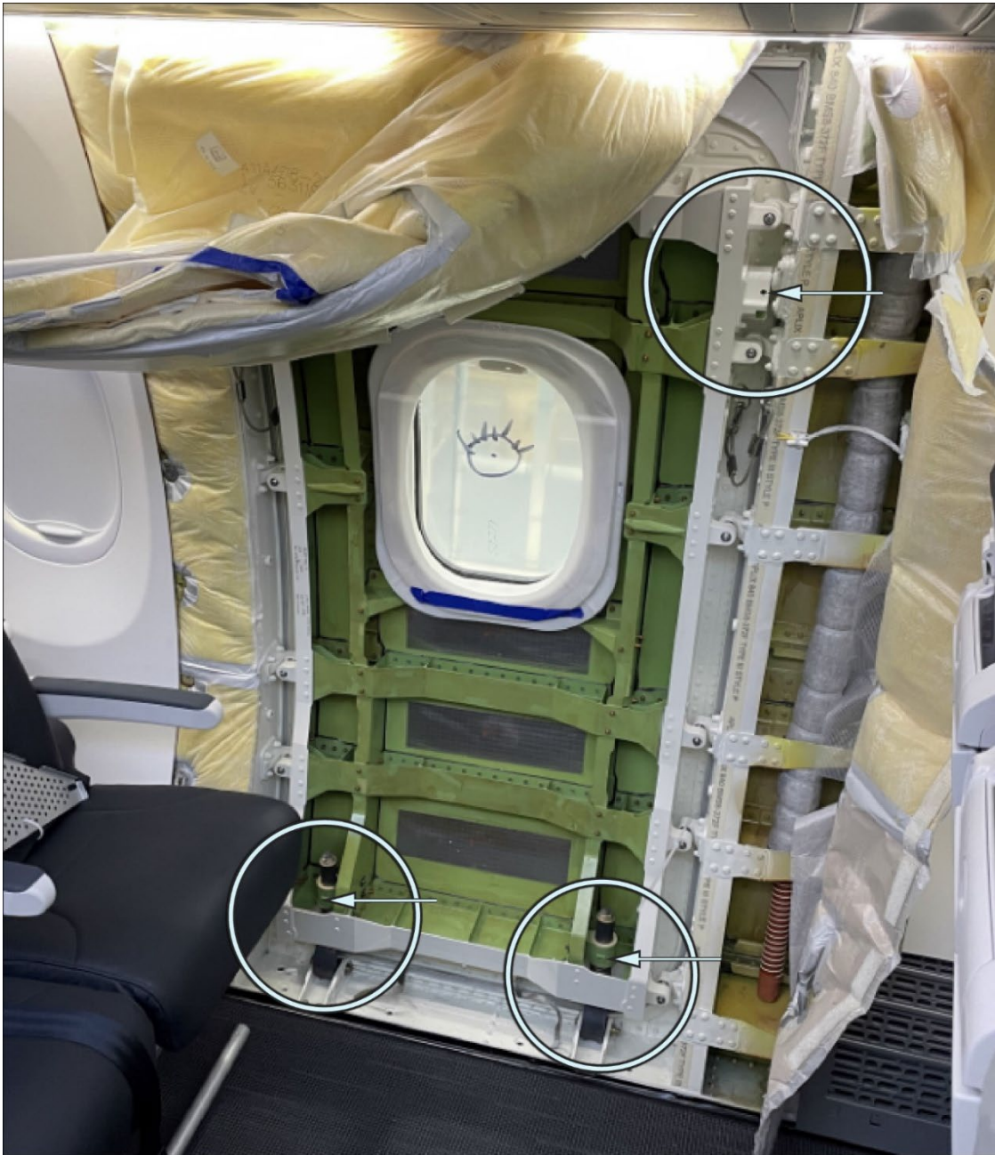
Figure 18. Photograph showing the left MED plug in the closed position with arrows indicating the locations of missing attachment hardware. Source: Boeing, cropped by NTSB.
