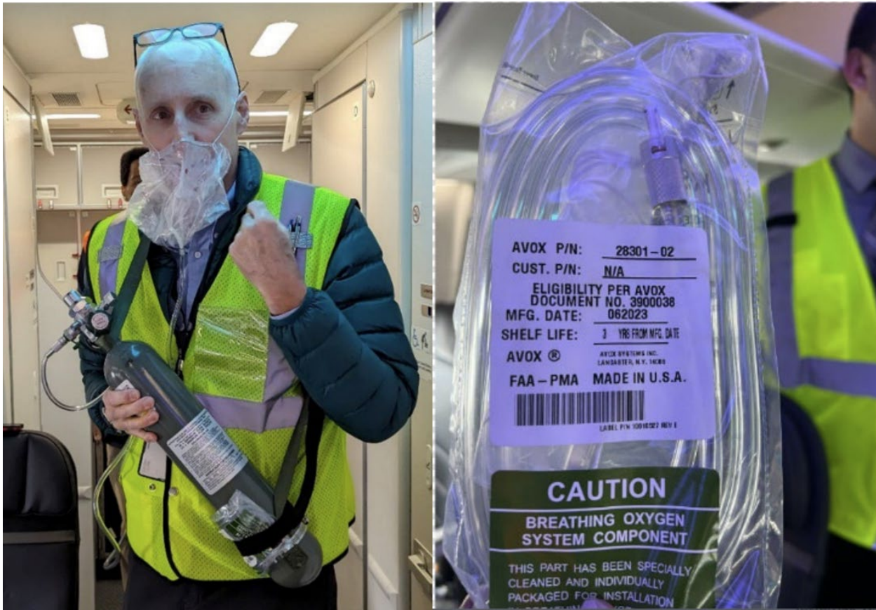
Figure 15. Side-by-side photographs of the mask and shoulder strap of a portable oxygen bottle on the accident airplane being worn (left) and a closeup of the packaging for a spare mask and tubing (right). (Source for both photographs: Boeing)
