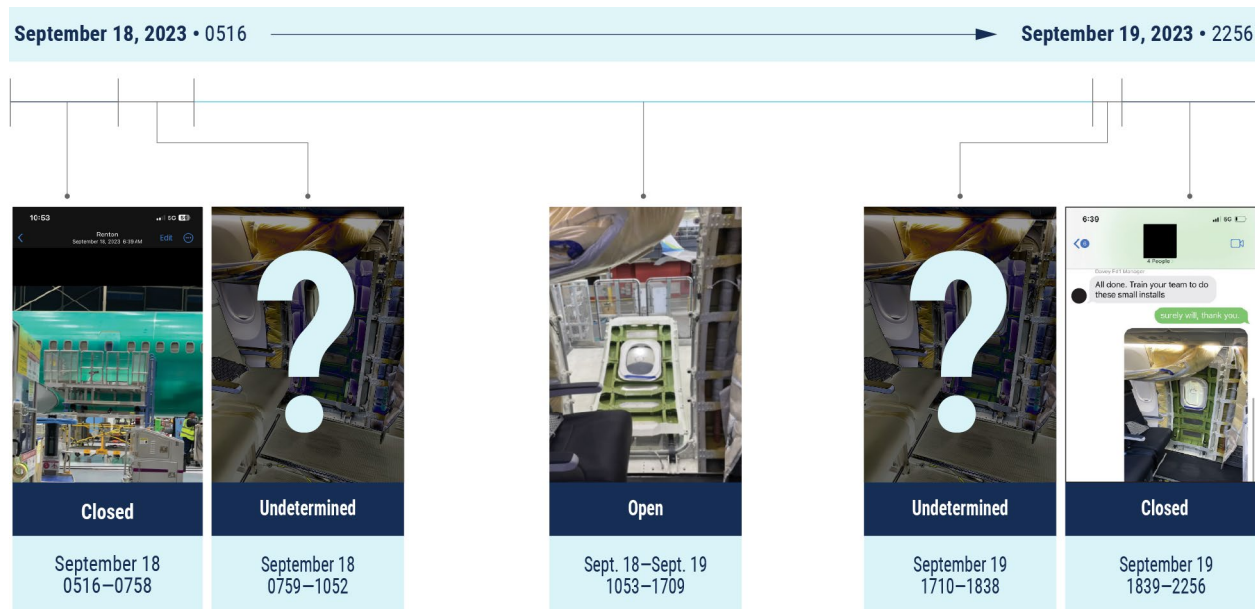
Figure 17. Timeline showing the periods for which evidence indicated the left MED plug was in a closed or open position and the periods for which its position was undetermined.
