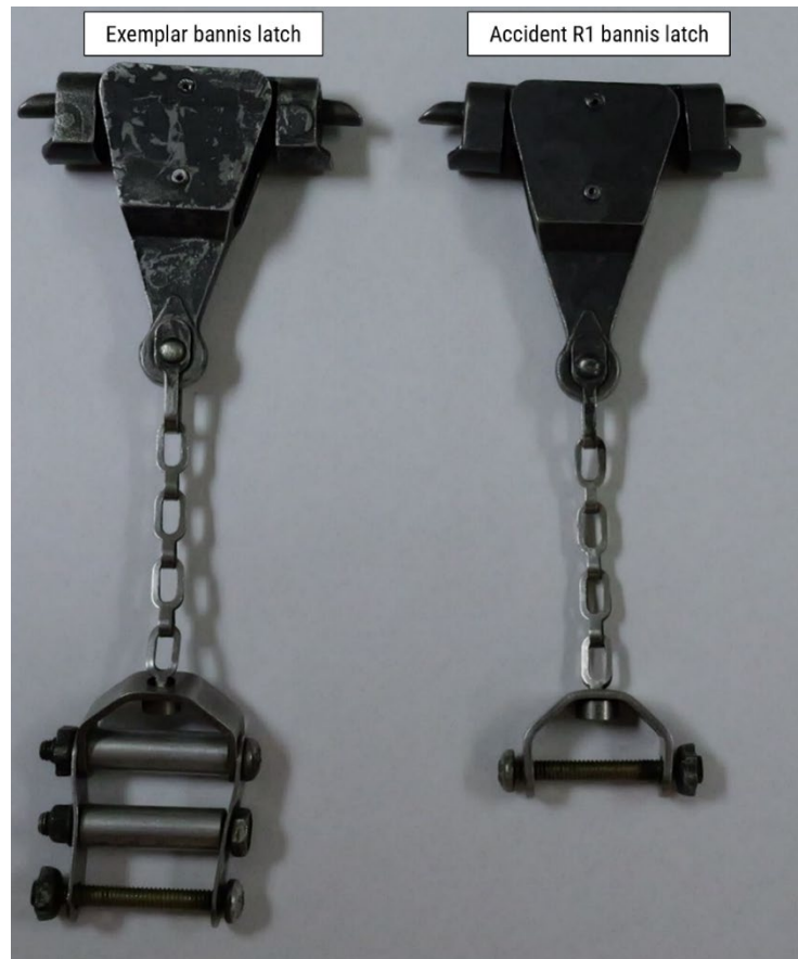
Figure 3. Exemplar bannis latch (left) with three links and accident airplane R1 bannis latch (right) with one link
