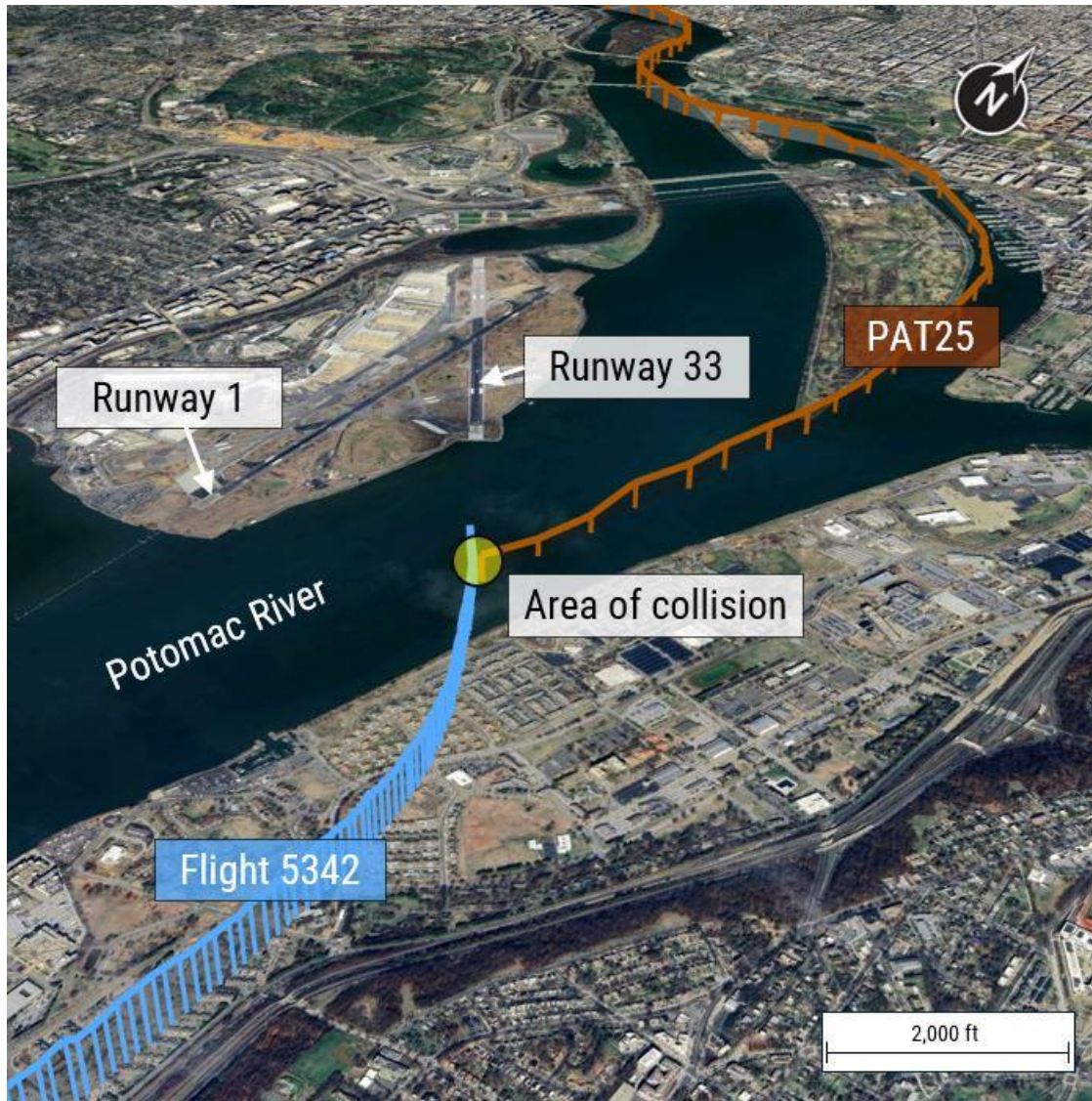
Figure 1. Google Earth image with preliminary ADS-B flight track for flight 5342 (blue line) and preliminary radar data for PAT25 (orange line).
