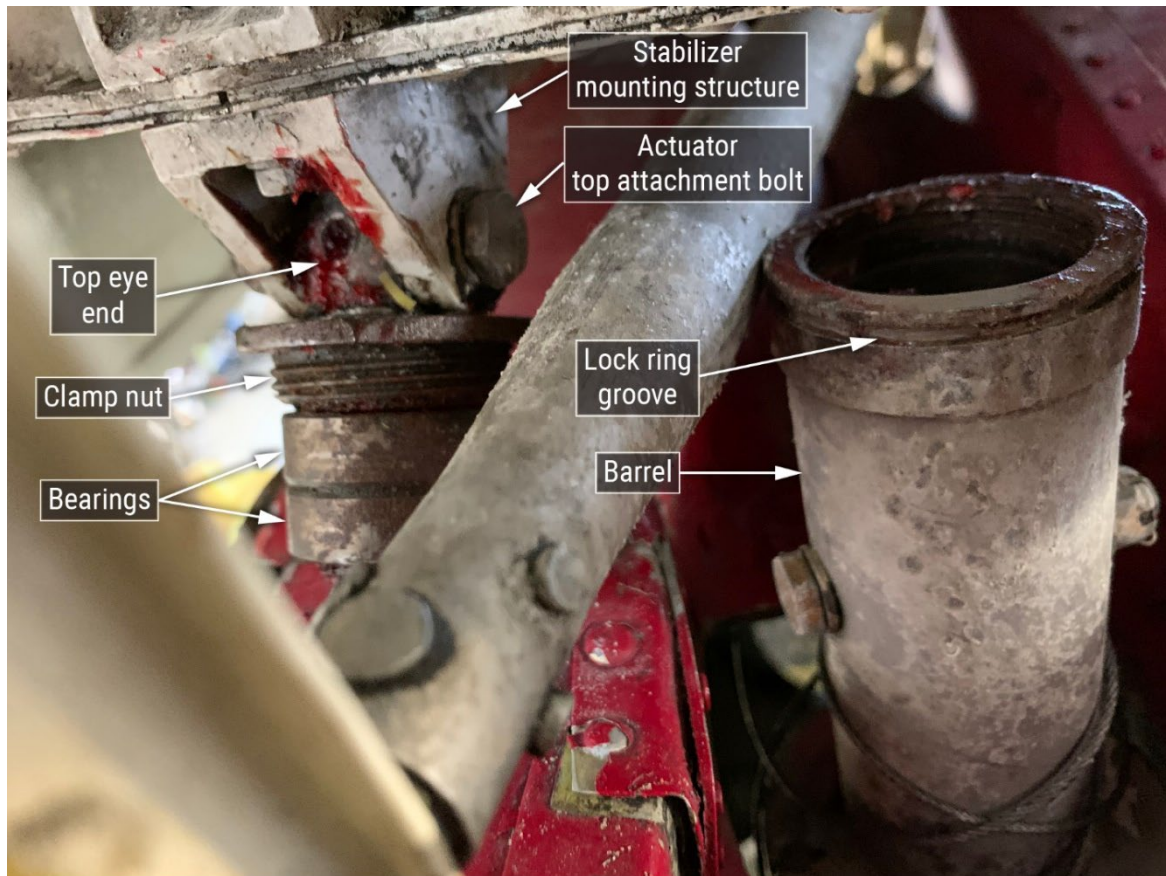
Figure 3. Clamp nut and barrel separation on accident airplane.
