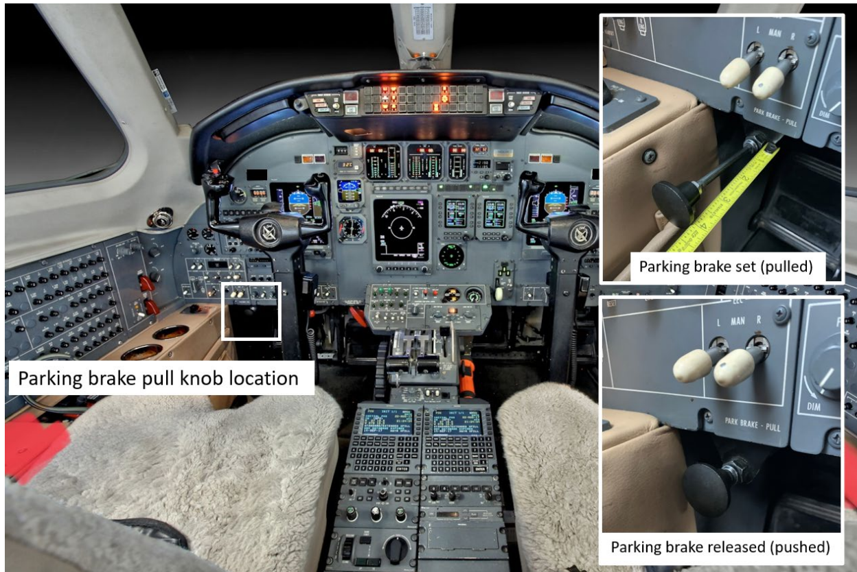
Figure 1. The location of the parking brake pull knob in a Cessna 560XL exemplar airplane (XLS model). (Source: Delta Private Jets)
