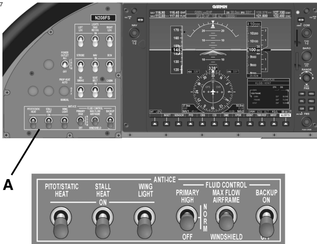
Figure 3. TKS ice protection system switches on the Model 208B pilot instrument panel. (Source: Model 208B POH)
