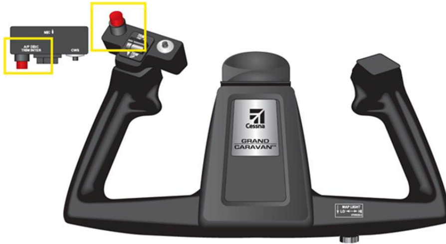
Figure 4. Model 208B control wheel with the autopilot disconnect button highlighted. (Source: Textron Aviation)
