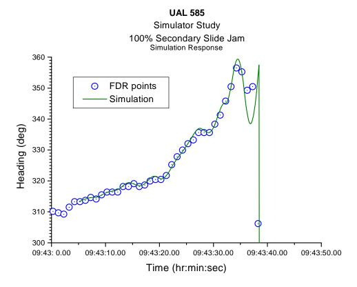
Figure 22d. Heading data for United flight 585.
