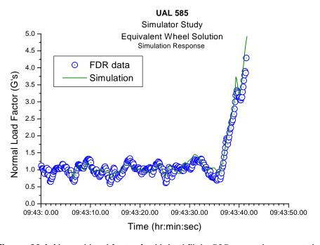
**Figure 23d.** Normal load factor for United flight 585 assuming a sustained equivalent control wheel input.
