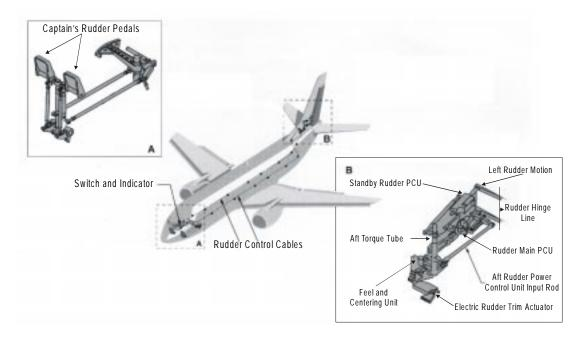
Figure 6. Boeing 737 rudder system.
