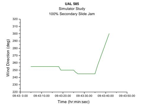
Figure 22j. Wind direction for United flight 585.
