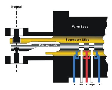
**Figure 14.** Normal operation of the 737 PCU servo valve with slides in the neutral position (no jam).
