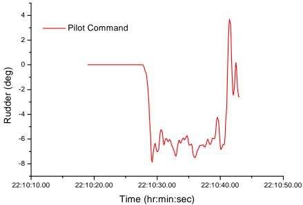
**Figure 27b.** Boeing's kinematic rudder for Eastwind flight 517 with pilot command and no yaw damper activity.
