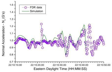
Figure 25f. Normal acceleration data for Eastwind flight 517.
