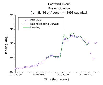
Figure 28b. Eastwind flight 517 heading data according to Boeing's scenario.
