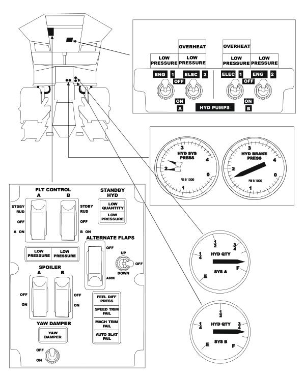
Figure 2. Boeing 737 hydraulic system panel.
