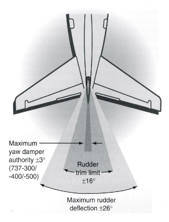
**Note:** The maximum 737 rudder deflection that the yaw damper can command is only a small portion of the total rudder travel. Yaw damper limits of the 737-100 and -200 can be 2, 3, or  $4^{\circ}$ , depending upon the installation.
