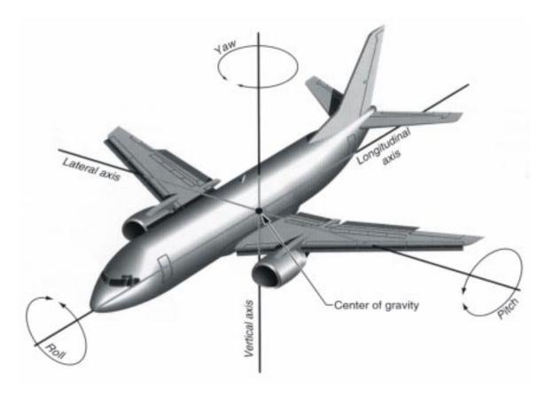
Figure 3. Three axes of motion.
