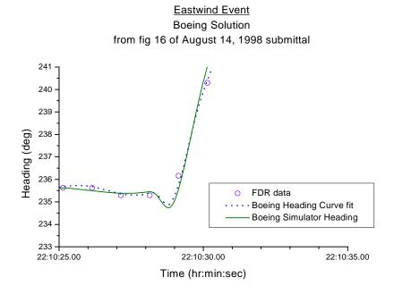
Figure 32. Boeing's curve fit of the FDR heading data from Eastwind flight 517.
