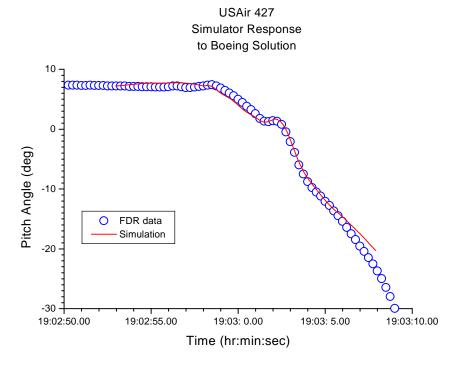
**Figure 21c.** Derived pitch angle for USAir flight 427 using Boeing's kinematic analysis.
