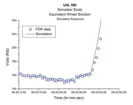
**Figure 23e.** Calibrated airspeed for United flight 585 assuming a sustained equivalent control wheel input.
