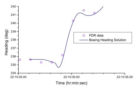
**Figure 26a.** Eastwind flight 517 heading data according to Boeing's scenario.
