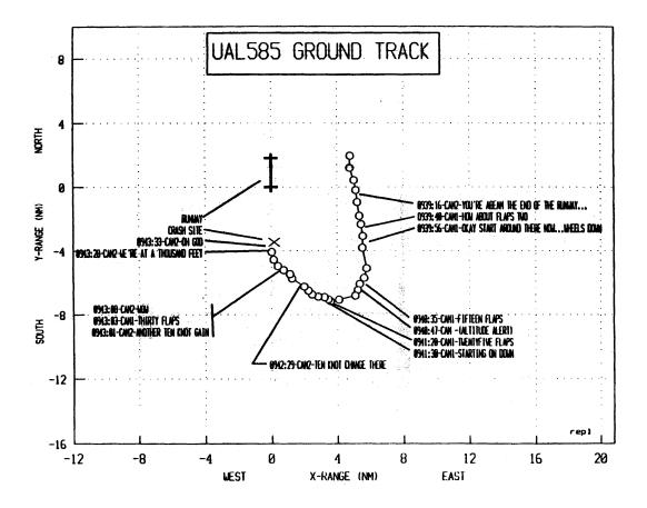
Figure 11. Ground track of United flight 585.
