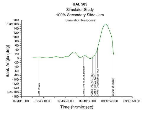
Figure 22g. Bank angle data for United flight 585.
