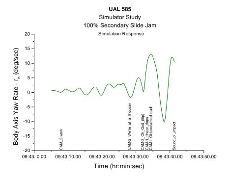
Figure 22i. Yaw rate for United flight 585.
