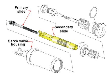
Figure 10. Boeing 737 main rudder PCU servo valve.
