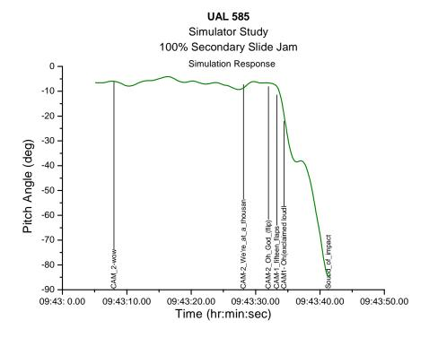
Figure 22f. Pitch angle data for United flight 585.
