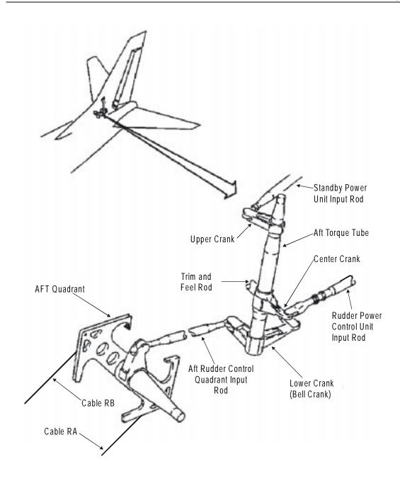
Figure 6a. Detailed view of 737 aft rudder system controls and linkages.
