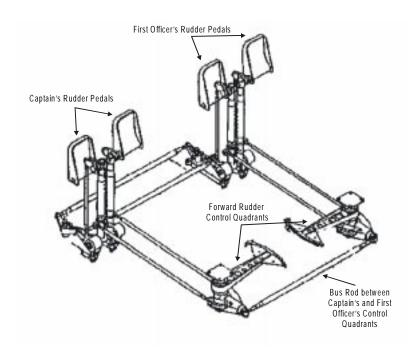
Figure 12. Rudder pedal assemblies as installed on the USAir flight 427 airplane.
