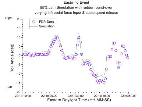
Figure 25e. Roll angle data for Eastwind flight 517.
