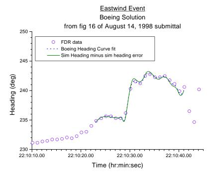
Figure 28d. Eastwind flight 517 corrected heading according to Boeing's scenario.
