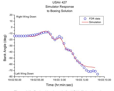
**Figure 21b.** Derived bank angle for USAir flight 427 using Boeing's kinematic analysis.
