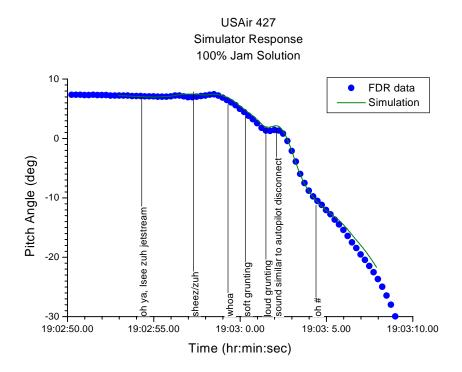
Figure 18f. Pitch angle data for USAir flight 427.
