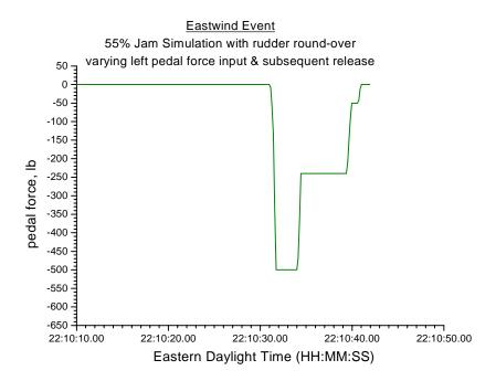
Figure 25c. Pilot rudder pedal force for Eastwind flight 517.
