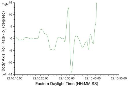
Figure 25j. Roll rate for Eastwind flight 517.
