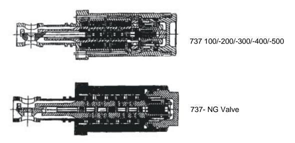
Figure 31. Parker's 1998 redesigned servo valve for 737 airplanes.
