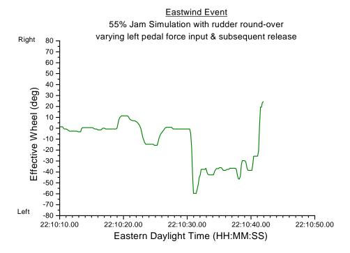
Figure 25b. Control wheel positions for Eastwind flight 517.
