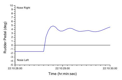
**Figure 26b.** Eastwind flight 517 pilot rudder pedal force according to Boeing's scenario.
