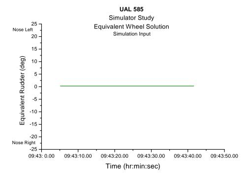
**Figure 23a.** Rudder surface positions for United flight 585 assuming a sustained equivalent control wheel input.
