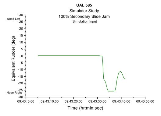
Figure 22b. Rudder surface positions for United flight 585.
