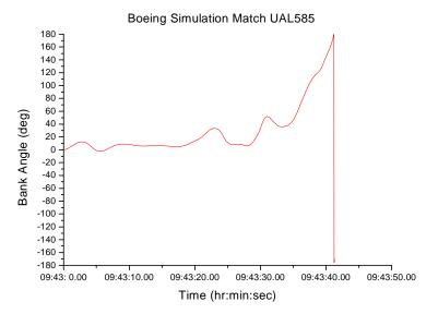
**Figure 24e.** United flight 585 bank angle data according to Boeing's new rotor model.
