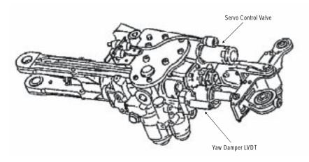
Figure 7. Boeing 737 main rudder PCU.
