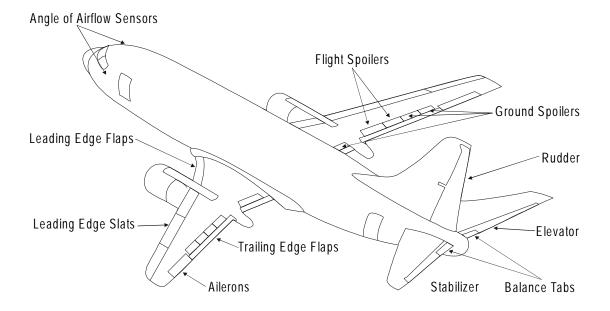
Figure 4. Boeing 737 flight control surface locations.
