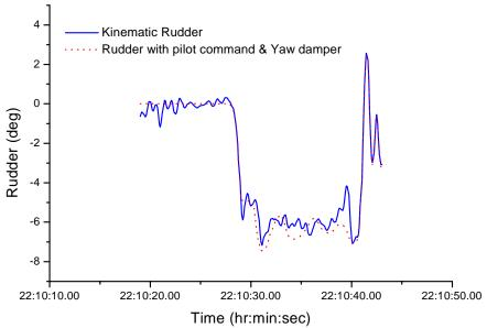
**Figure 27a.** Boeing's kinematic rudder for Eastwind flight 517 and rudder with pilot command and yaw damper activity.
