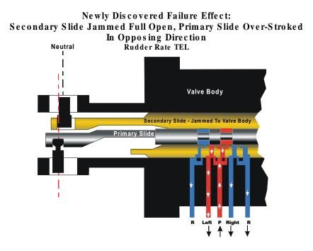
**Figure 17.** PCU servo valve with the secondary slide jammed to the servo valve housing and the primary slide in the overtravel condition.
