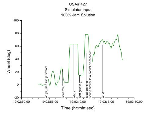
Figure 18c. Control wheel positions for USAir flight 427.
