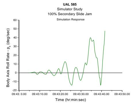
Figure 22h. Roll rate for United flight 585.
