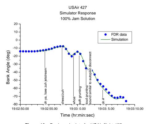
Figure 18e. Bank angle data for USAir flight 427.
