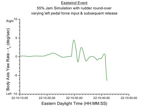
Figure 25i. Yaw rate for Eastwind flight 517.
