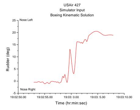
**Figure 19.** USAir flight 427 rudder surface positions resulting from Boeing's kinematic analysis.
