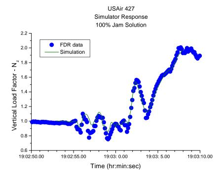
Figure 18g. Vertical acceleration data for USAir flight 427.
