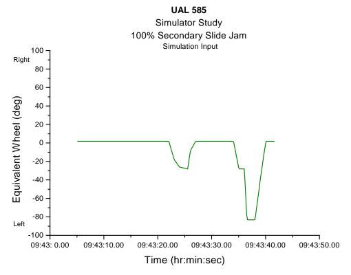
Figure 22c. Control wheel positions for United flight 585.
