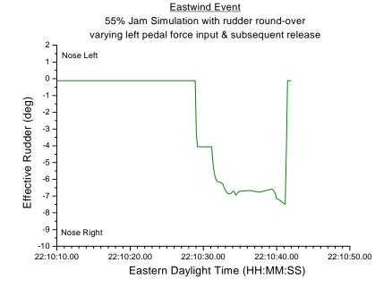
Figure 25d. Rudder surface positions for Eastwind flight 517.
