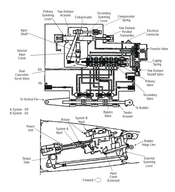
Figure 8. Boeing 737 main rudder PCU schematic and installation.
