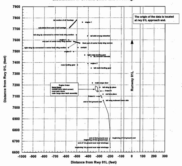
Distribution of Ground Scars and Wreckage
