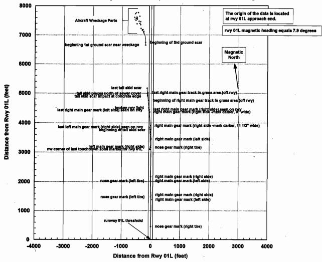
Distribution of Surveyed Ground Marks, Ground Scars and Wreckage
