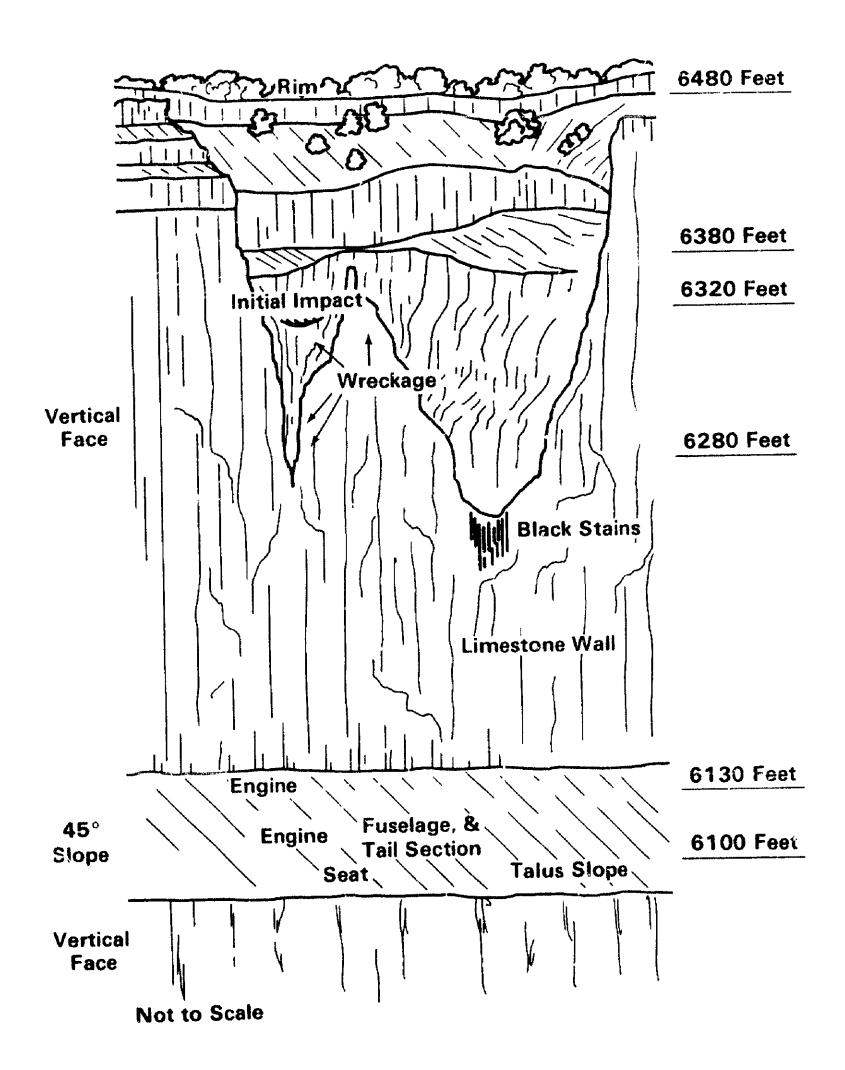
Figure 2.—Wreckage diagram.
