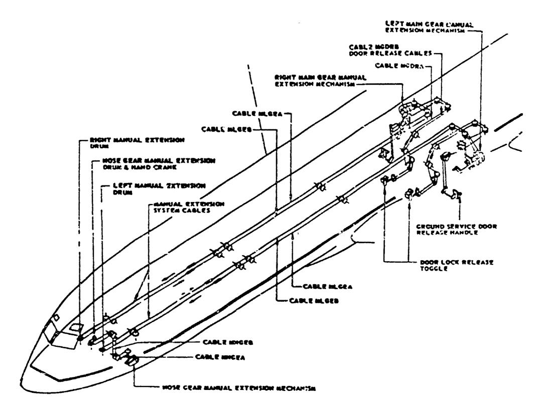
Figure 1.—Manual gear extension system.
