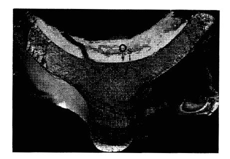
Figure 4. Portion of inboard fracture surface removed for detailed fractographic examination. Arrow "0" denotes main origin and arrow "S" locates secondary origin while dashed lines indicate approximate extent of fatigue propagation from these origins.
