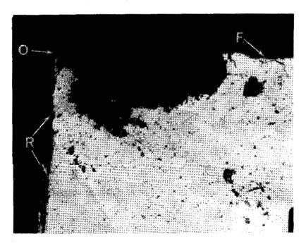
Figure 8. Longitudinal metallographic microsection through the main origin area showing the discontinuity in profile. Arrows "R" and "F" indicate the radius and fracture profile respectively. X375 Kellers etch
