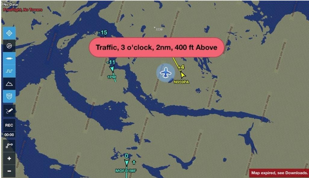
**Figure 5.** Example of a ForeFlight visual traffic alert with a traffic pop-up display.
