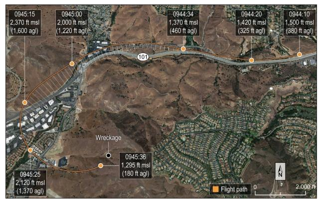
Figure 4. Accident flight's climb, left turns, rapid descent, and wreckage location.
