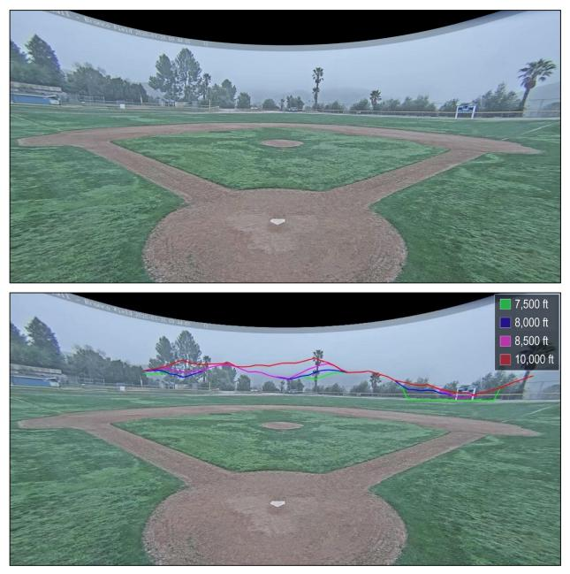
**Figure 12.** A distortion-corrected image from video captured by Camera A at the accident time (top). Terrain outline curves are superimposed on the same image for the specified computed visibility ranges (bottom).
