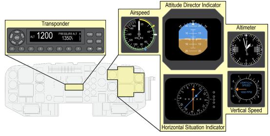
Figure 6. Exemplar instruments and transponder.
