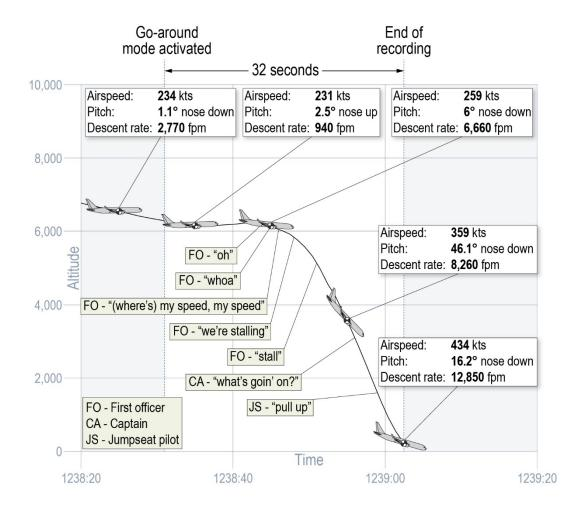
Figure 1. Selected airplane parameters and crew statements during final seconds of flight.8
