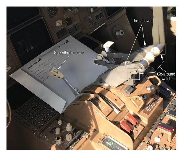
**Figure 7.** Locations of thrust levers, go-around switches, and speedbrake lever in an exemplar Boeing 767 airplane.
