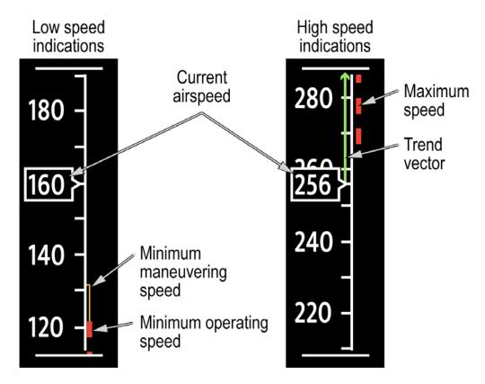
Figure 4. Exemplar airspeed tape indications.
