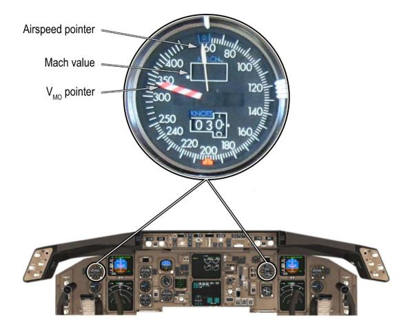
Figure 5. Exemplar conventional airspeed indicator.
