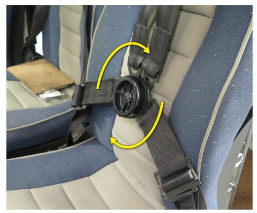
Figure 9. Exemplar four-point system with a rotary buckle.
