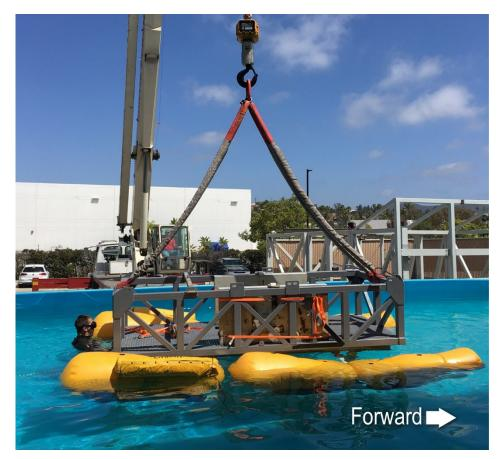
Figure 19. A test rig with partially, symmetrically inflated floats is shown suspended by a crane and lowered into a pool.
