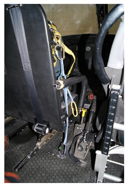
Figure 16. Front passenger's tether (attached to exemplar occupant) routed under the armrest.
