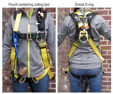
**Figure 10.** Front and rear views of a person wearing an exemplar yellow fall-protection harness with a pouch containing a cutting tool attached to the upper left shoulder strap.
