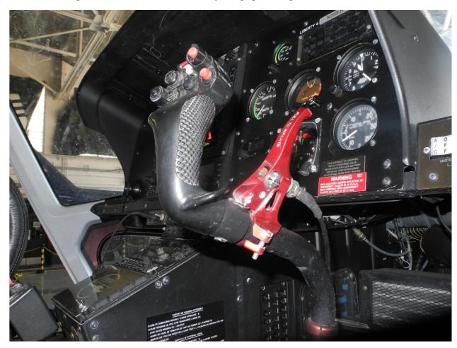
Figure 6. Float activation handle (red) installed on the accident helicopter's cyclic control.
