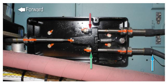
Figure 8. View inside the junction box for the accident helicopter's emergency flotation system.
