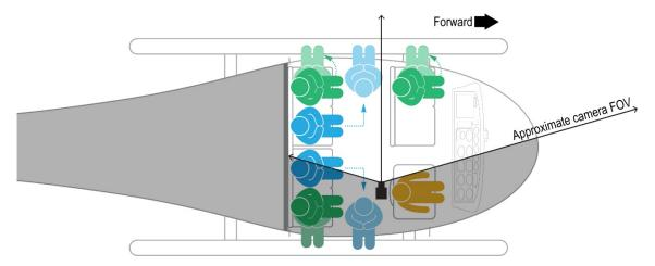
Figure 17. Diagram showing ceiling-mounted camera's approximate FOV.
